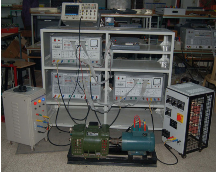
Fig. 12.5 Schematic of the experimental setup of matrix converter interfaced PMSG for wind energy conversion system
