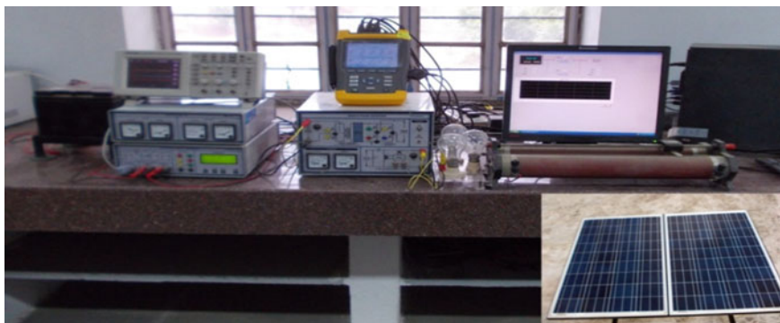
Fig. 13.8 Hardware structure of proposed grid PV system
