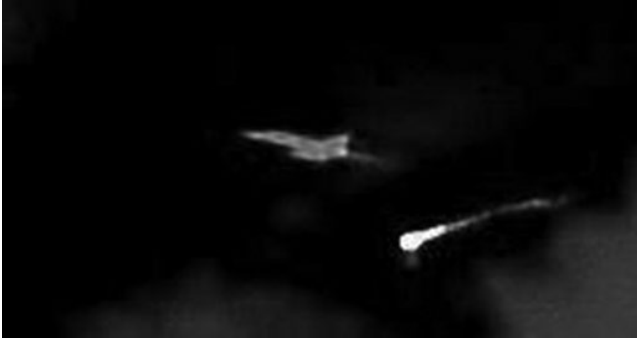
Figure 11.47 Thermal image of the target aircraft and a flare launched by it seen in the 3–5 \mu\text{m} band by a single colour IR-guided missile.
