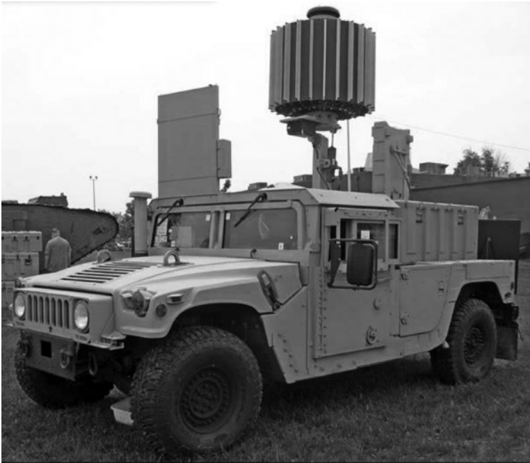
Figure 3.41 AN/TPQ-50 counter fire radar. (Source: Courtesy of Major Linda Wade, US Army.)
