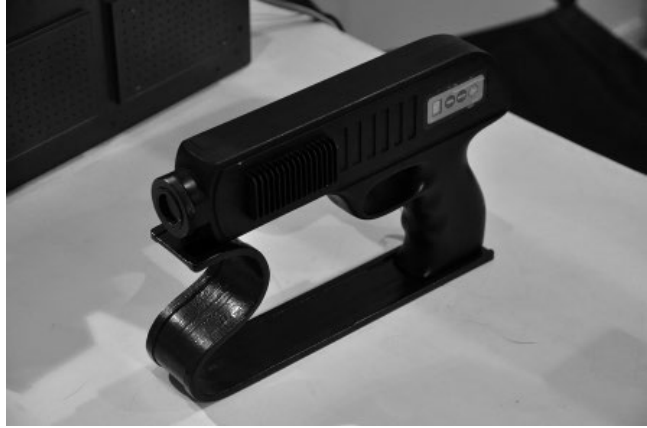
Figure 12.38 Hand-held laser dazzler developed by LASTECH DRDO. (Source: Biswarup Ganguly, https://commons.wikimedia.org/wiki/File:Laser_Dazzler_-_DRDO_-_Pride_of_India_-_Exhibition_-_100th_Indian_Science_Congress_-_Kolkata_2013-01-03_2560.JPG . CC BY 3.0.)
