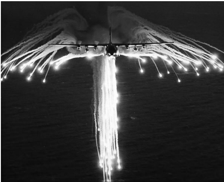
Figure 6.18 Ejection and ignition of a typical pyrotechnic infrared decoy flare. (Source: TidusTia, https://commons.wikimedia.org/wiki/File:C-130_Hercules_10.jpg .CC BY-SA 3.0.)
