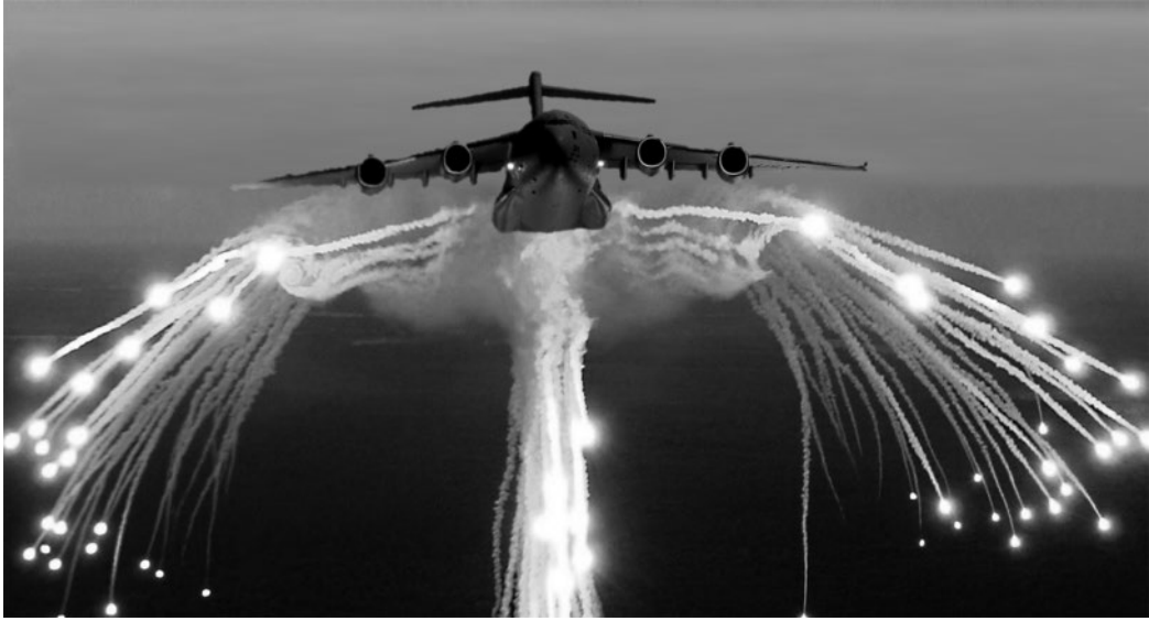
Figure 6.22 Infrared flares deployed from AN/ALE-47 CMDS installed on a C-17 Globemaster-III aircraft.
