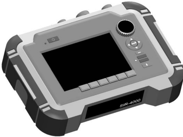
Figure 3.33 SIR-4000 GPR Control Unit.
