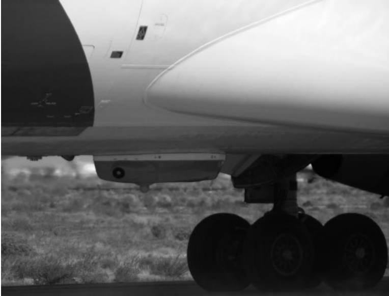
Figure 6.41 GUARDIAN DIRCM pod. (Source: Alan Radecki Akradecki, https://commons.wikimedia.org/wiki/File:Fedex-md11-N525FE-051109-08-16.jpg . CC BY-SA 3.0.)
