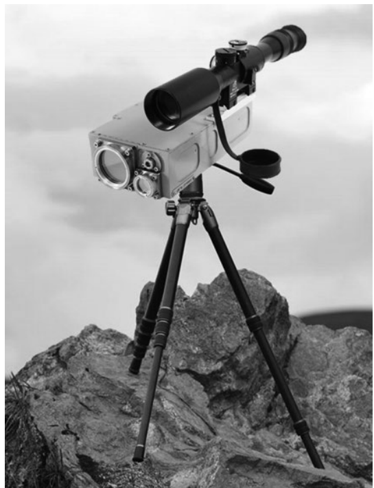
Figure 10.11 DL-20 laser range finder module.
