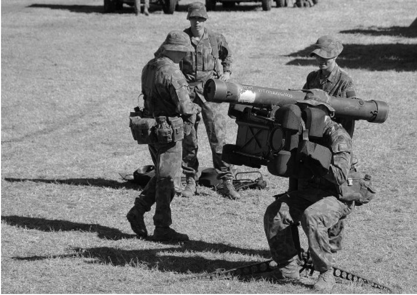
Figure 11.8 RBS-70 NG laser beam rider MANPADS. (Source: Courtesy of the US Navy.)
