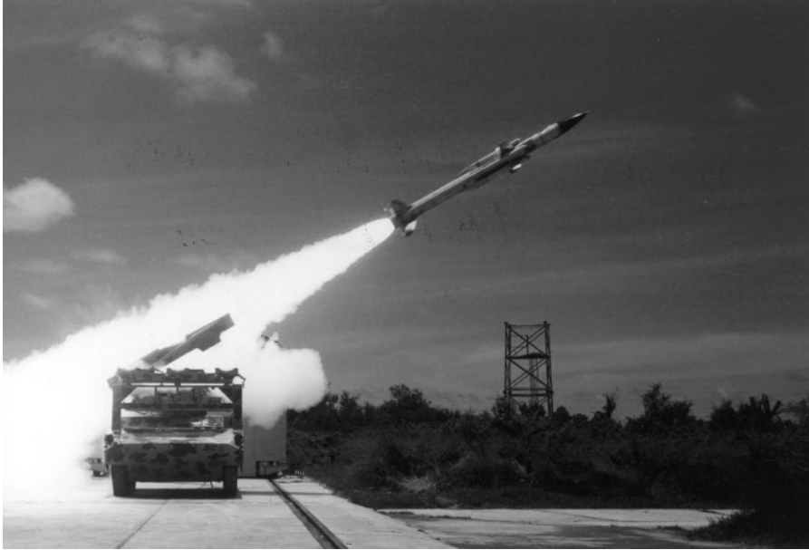
Figure 11.70 Akash medium range surface-to-air missile. (Source: Frontier India Defense and Strategic News Service, https://commons.wikimedia.org/wiki/File:Akash_SAM.jpg . CC BY-SA 2.5 IN.)
