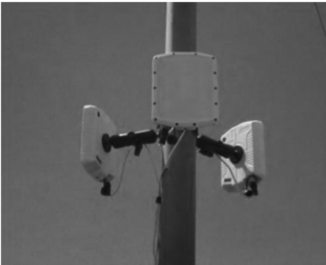
Figure 3.13 Three C20 radars to give 360° coverage. (Source: Courtesy of SpotterRF.)
