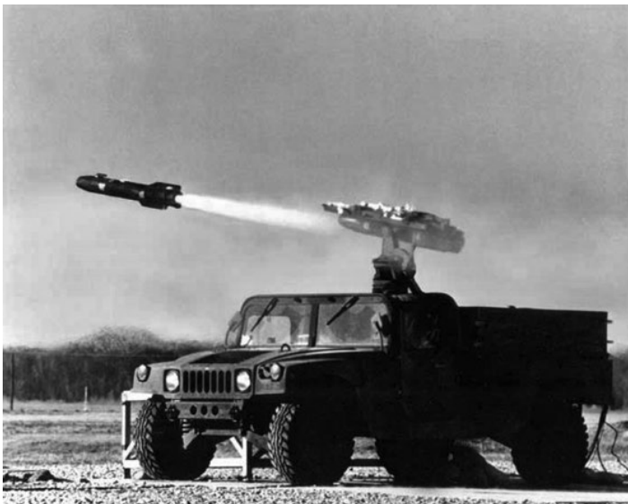
Figure 11.30 Hellfire-II fired from a land vehicle. (Source: Courtesy of the US Army.)
