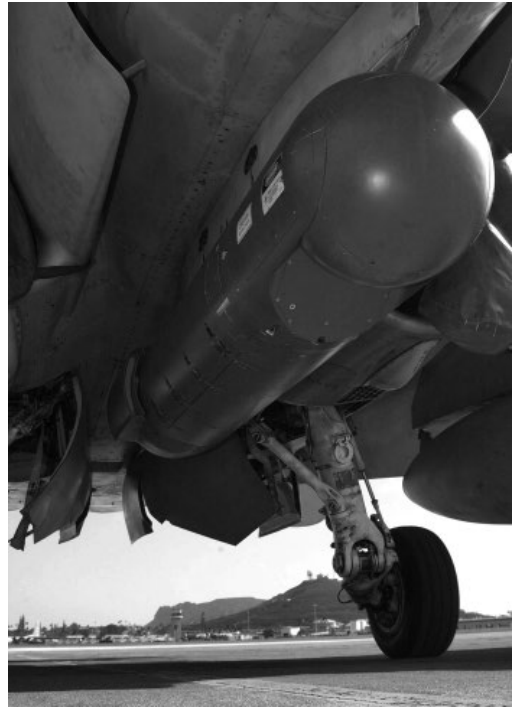
Figure 10.34 LITENING targeting pod. (Source: Courtesy of the US Government.)
