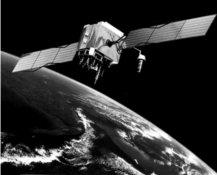
Figure 4.63 Flat solar panel on a three-axis stabilized satellite. (Source: Courtesy of NASA.)
