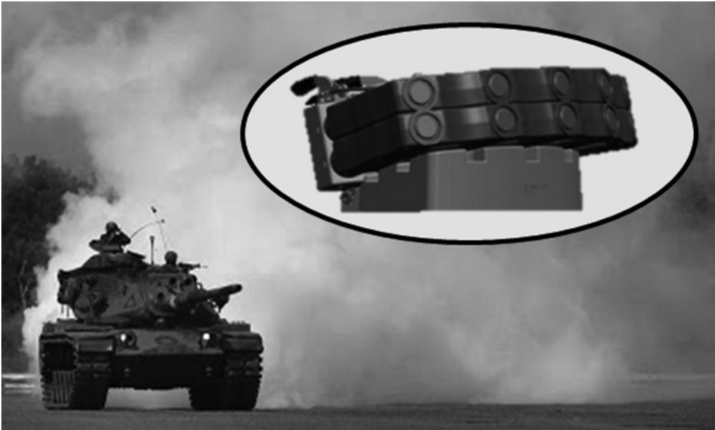
Figure 6.32 ROSY-L Rapid Obscuring System.
