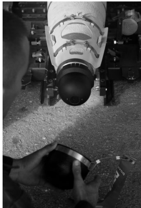
Figure 11.31 LJDAM integrated with an F-16C aircraft. (Source: Courtesy of the US Military.)
