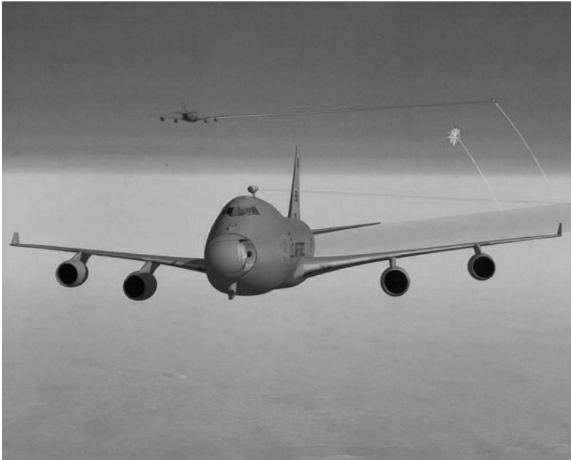
Figure 12.48 Airborne laser for ballistic missile defence. (Source: Courtesy of the US Airforce.)
