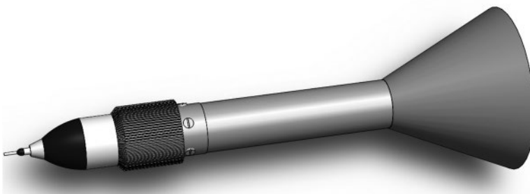
Figure 6.28 Ariel towed radar decoy.
