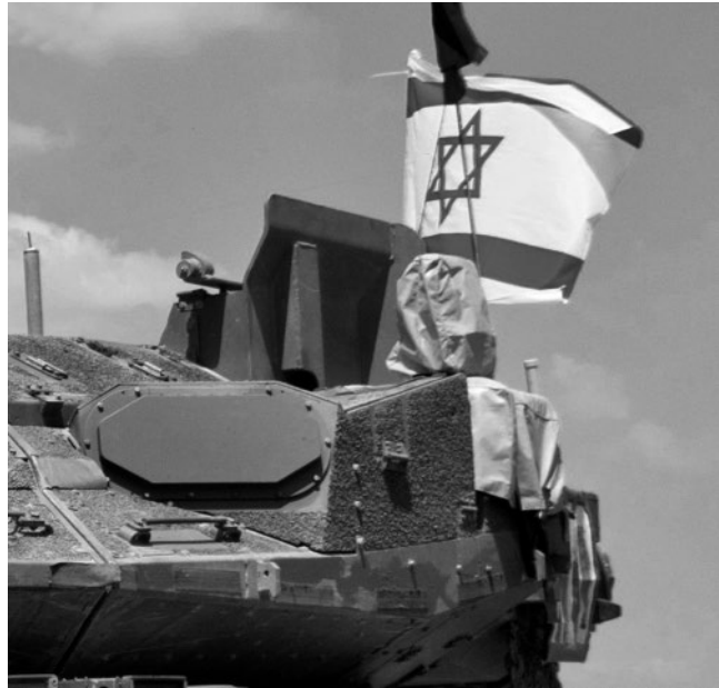
Figure 6.35 The Trophy Active Protection System. (Source: Zachi Evenor, https://commons.wikimedia.org/wiki/File:Trophy-APS--Merkava-4M-pic01-Zachi-Evenor_(cropped).jpg , CC BY 3.0.)
