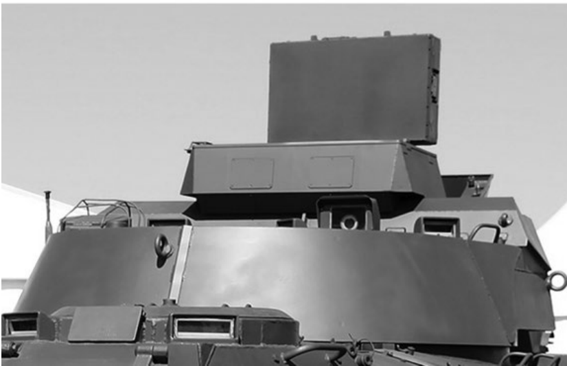
Figure 3.18 (a) NAR-10M1 surveillance radar mounted on an MT-LB vehicle. (b) Close up view. (Part (a) Source: Vitaly V. Kuzmin, http://www.vitalykuzmin.net/Copyright-policy.CC BY-SA 4.0. )
