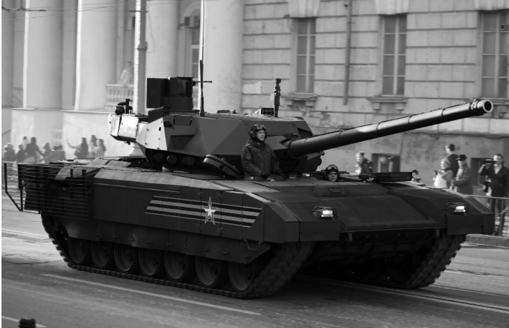
Figure 6.48 T-14 Armata Main Battle Tank. (Source: Vitaly V. Kuzmin, https://commons.wikimedia.org/wiki/File:VDayRehearsal05052016-28.jpg .CC BY-SA 4.0.)
