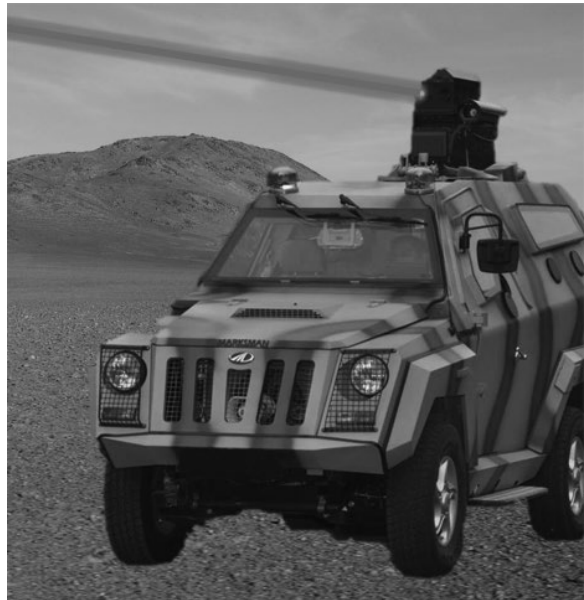
Figure 12.39 Crowd control laser dazzler mounted on a Mahindra Marksman Light Armoured Vehicle.
