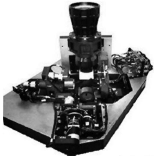
Figure 11.62 IR target generator from CI Systems, Israel.
