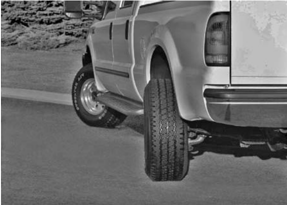
Figure 27.8 Four-wheel steering under low vehicle speed condition, where the front and rear wheels are in phase opposition (courtesy Delphi Corporation).
