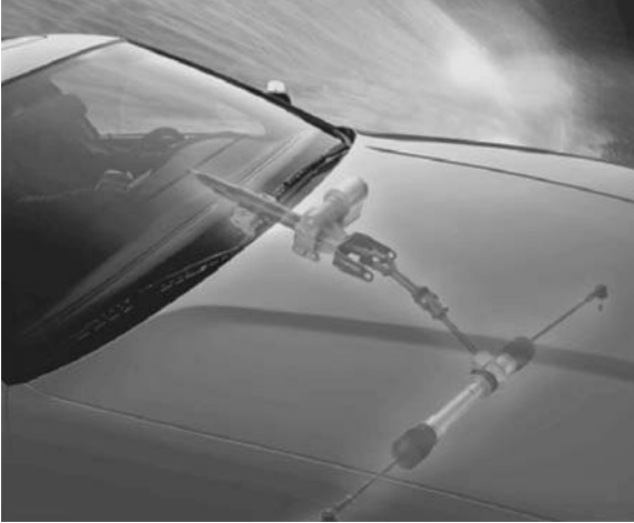
Figure 27.5 Mechanization of an electric power steering system (courtesy Delphi Corporation).
