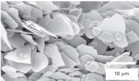
26.2 Photomicrograph of plate-like \text{Bi}_4\text{Ti}_3\text{O}_{12} particles prepared in molten KCl.
