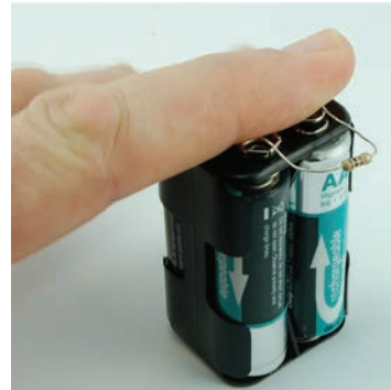
FIGURE 3-3 Making a resistor get hot
