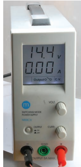
FIGURE 12-7 A lab power supply
