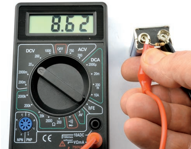
FIGURE 11-4 Testing a battery using a resistor and multimeter
