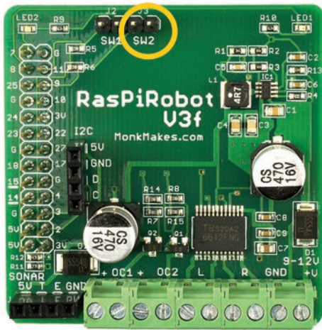
FIGURE 8-27 The SW2 contacts on the RasPiRobot Board V3
