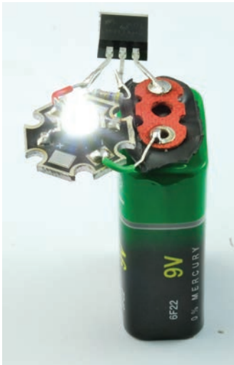
FIGURE 4-13 Emergency LED lighting
