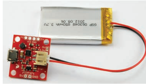
FIGURE 5-10 Combined LiPo charger and booster
