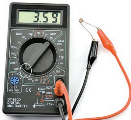
FIGURE 3-8 Measuring the LDR resistance
