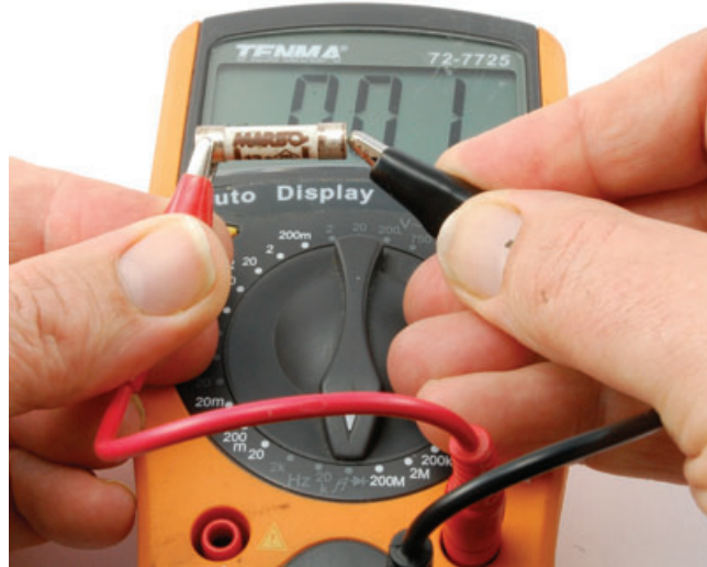
FIGURE 10-3 Testing a fuse with a multimeter
