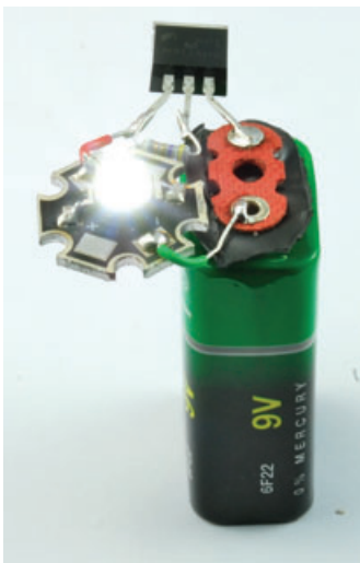
FIGURE 4-13 Emergency LED lighting
