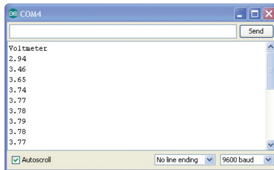
FIGURE 6-18 The Serial Monitor showing voltage at A3
