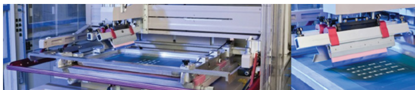
Figure 2.14 Screen printer using Clevios™ ink. (Reproduced with permission from Heraeus.)
