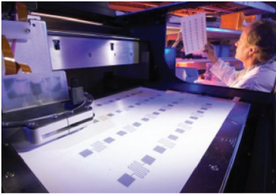
Figure 2.19 Inkjet printer using Clevios™ ink. (Reproduced with permission from Heraeus.)
