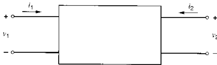
Figure 8.28 Circuit equivalent to that of Fig. 8.27 using a two-port representation of the feedback network.
