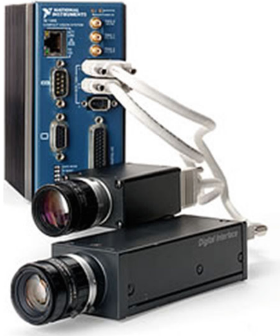
Fig. 2.10 NI compact vision system
