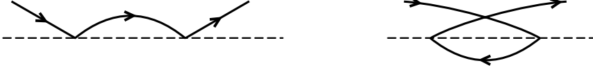
Fig. 24.10. Second-order processes of the s - d interaction. Time flows from left to right. The electron propagating backward in time corresponds to a hole
