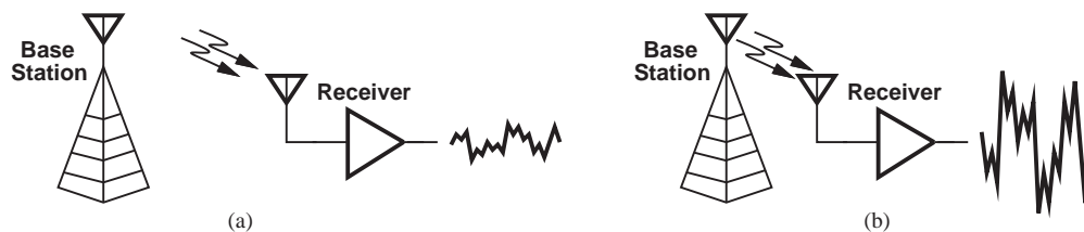
Figure 3.47 Signals received (a) far from or (b) near a base station.
