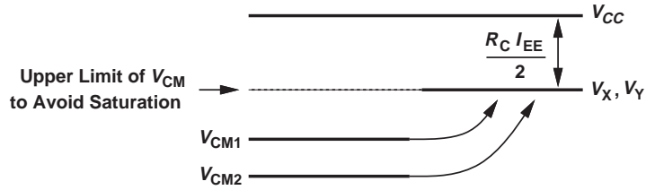
Figure 10.8 Effect of V_{CM1} and V_{CM2} at output.
