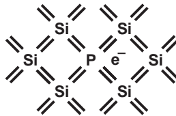
Figure 2.5 Loosely-attached electron with phosphorus doping.
