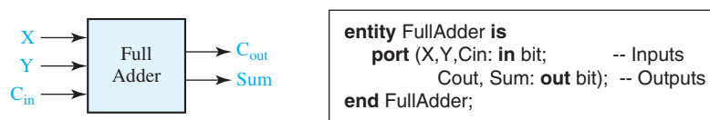
FIGURE 10-10 Entity Declaration for a Full Adder Module
