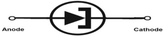
Fig. 2.18 Symbol of tunnel diode
