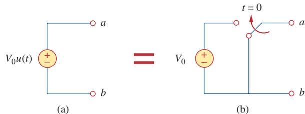
**Figure 7.25**(a) Voltage source of  $V_0 u(t)$ , (b) its equivalent circuit.
