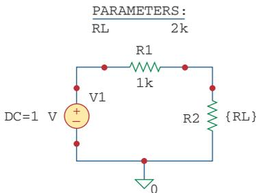
**Figure 4.56** Schematic for the circuit in Fig. 4.55.
