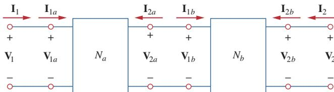
**Figure 19.41** Cascade connection of two two-port networks.
