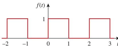
Figure 17.1 For Example 17.1; a square wave.
