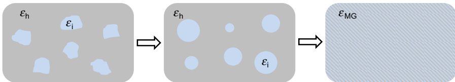
Figure 7.1 On the left is the microstructure under investigation, which is a two-phase medium with very small guest inclusions of unknown shapes and dielectric constant \epsilon_i dispersed in a continuous host medium with permittivity \epsilon_h . On the central panel is the Maxwell Garnett “view” of the material on the left, in which the inclusions are described as small spheres of dielectric constant \epsilon_i . On the right is Maxwell Garnett homogenization, with effective permittivity \epsilon_{MG} .
