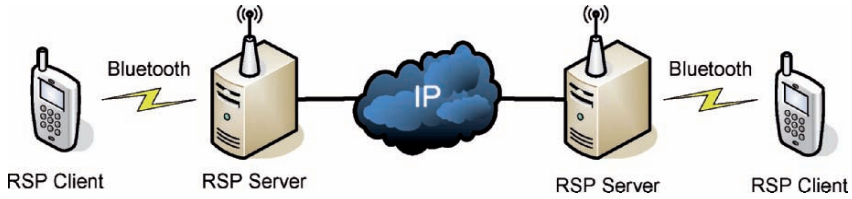
Figure 12.7. Proof of concept setup of Bluetooth-IP.
