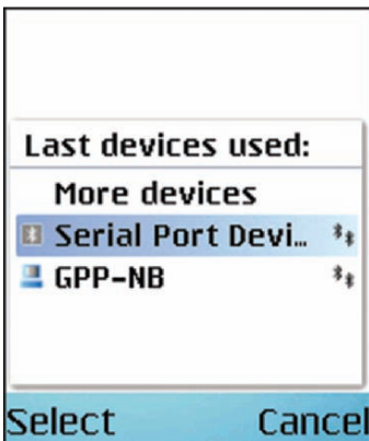
(c) Select the device to connect to. In this case the sensor is represented by the “Serial Port Device” entry in the list of Bluetooth devices found.
