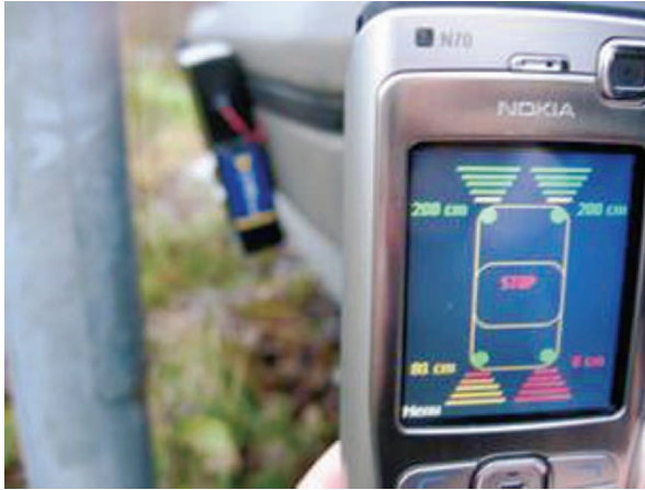
Figure 22.1. This picture shows the sensors plugged on the car and the screen of the phone during the test phase of the application.
