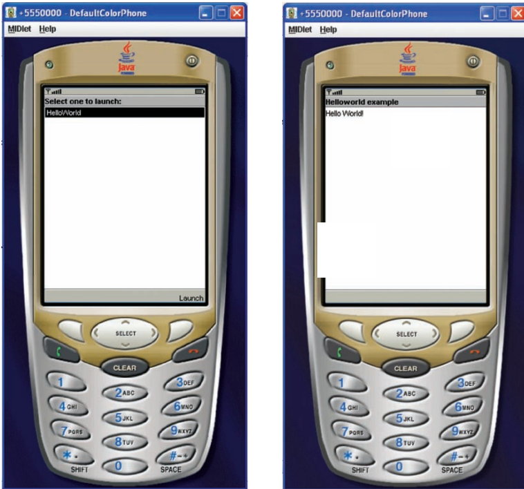
(a) The names of available MIDlets are listed, but the project is not running; pressing the “Launch” key, the application starts. (b) HelloWorld example running.
