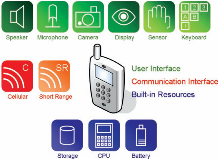
Figure 1.4. A mobile device broken up into the several capabilities grouped into the user interface, communication interface, and the built-in resources.
