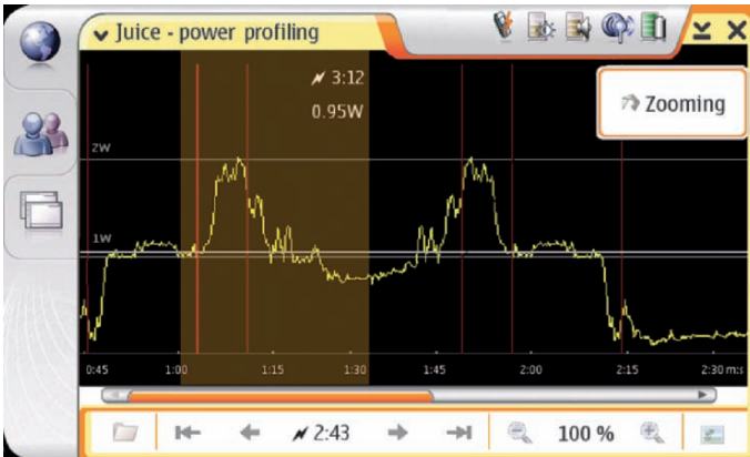
Figure 25.5. Concept drawing of Juice running on the Maemo platform. The bigger display area and pen input available in Internet tablets allow for an improved interface for power consumption analysis.
