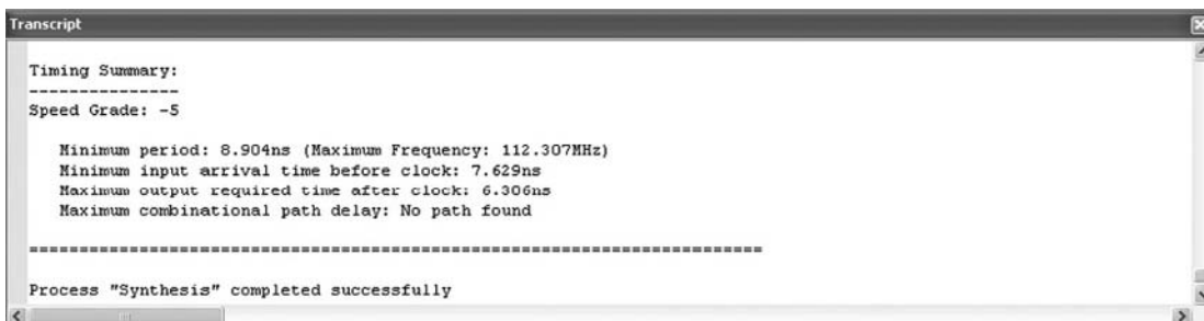
Figure 6–24: Successful Synthesis Shown in Transcript Window (Material based on or adapted from figures and text owned by Xilinx, Inc., courtesy of Xilinx, Inc. Copyright © Xilinx 1995–2008 used in Xilinx ISE WebPack™ software version 10.1.)
