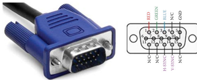
FIGURE 8.14 Picture and pin details of a VGA DB15 connector.
