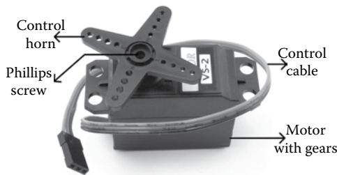
FIGURE 9.9 Picture of a servo motor with label for its important parts.
