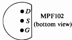
FIGURE 18-2 Pin configuration of MPF102 JFET.
