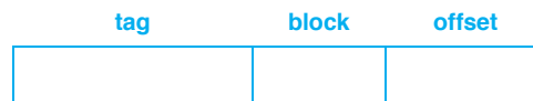
Figure 12.9 Illustration of how using powers of two allows a cache to divide a memory address into three separate fields that correspond to a tag, a block number, and a byte offset within the block.
