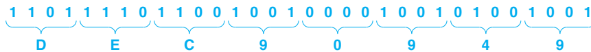
Figure 3.5 Illustration of the relationship between binary and hexadecimal. Each hex digit represents four bits.
