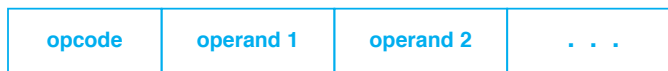
Figure 5.1 The general instruction format that many processors use. The opcode at the beginning of an instruction determines exactly which operands follow.
