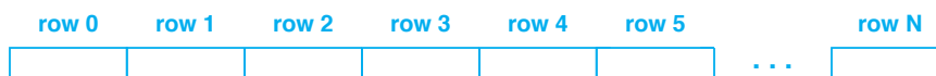
Figure 13.13 An illustration of a two-dimensional array stored in row-major order. A row is contiguous in memory.
