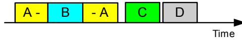
Fig. 3. Pre-emptive scheduling of Task A and Task B in the system shown in Fig. 2: Task B, here, is assigned a higher priority (Nahas, 2008).
