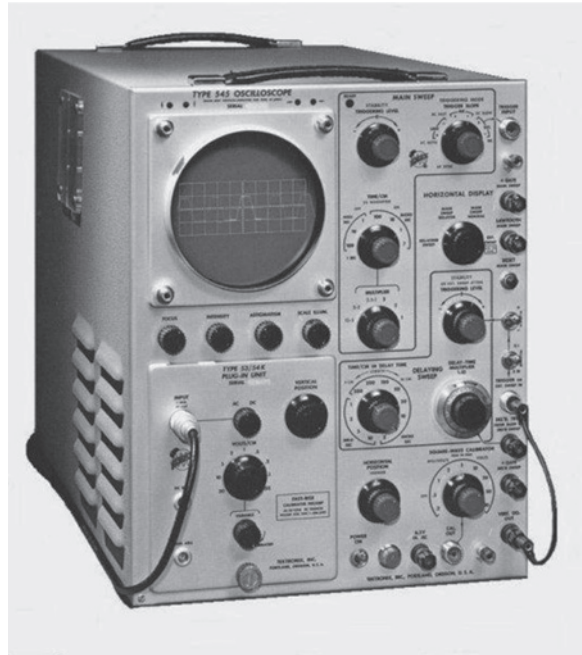
Figure 1.33: Tektronix introduced the 545 scope back in the dark ages; a half-century later, many are still going strong. Replace a tube from time to time and these might last forever. About the size of a two-drawer file cabinet and weighing almost 100 pounds, they're still favored by Luddites and analog designers.
