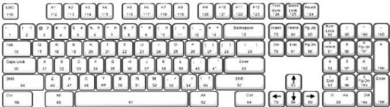
Figure 7.28 Standard 104-key Keyboard and Key Number
