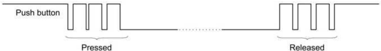
Figure 7.1 Contact Bounce in a Pushbutton
