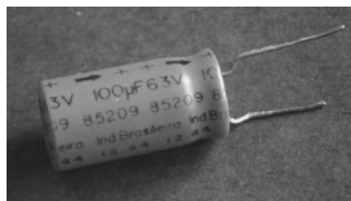
Figure 1.2. Symbol for the electrolytic capacitor (left), where one side must be more positive than the other side. The negative plate is drawn curved. On the right is a photo of an electrolytic capacitor in its characteristic cylindrical can shape. Notice that the positive end is clearly marked. Other styles have the negative end marked.
