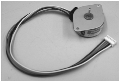
Figure 5.38. View of a stepper motor. It has a series of coils that, when energized, lock the motor shaft in position. Energizing a different set of coils makes the motor step in to a new position.
