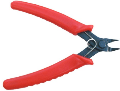
Figure 13-3: Diagonal cutters trim wire ends flush to the surface.
