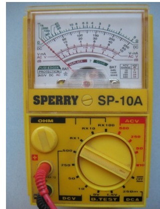
Figure 16-4: This circa-1980s analog multimeter uses a needle to indicate voltage, current, and other values.
