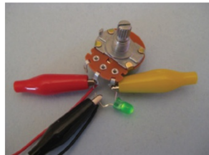
Figure 5-14: A resistor in series with a potentiometer ensures that current to the LED is restricted even if the pot is dialed down to zero ohms. Without that resistor, the LED is toast.
