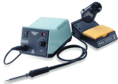
Figure 13-2: Some soldering iron models are temperature-adjustable and come with their own stands.
