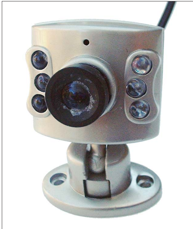
Figure 15-7: This miniature camera can see in the dark, thanks to its six infrared light-emitting diodes (IR LEDs).
