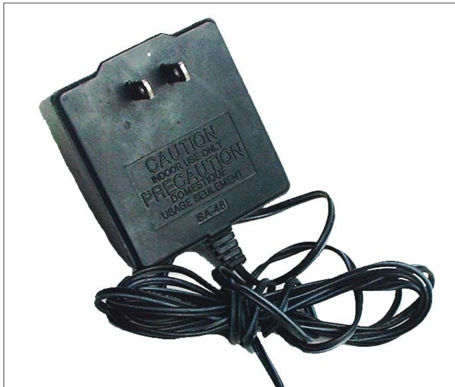
Figure 8-5: A plug-in wall transformer shields you from exposed AC house current.
