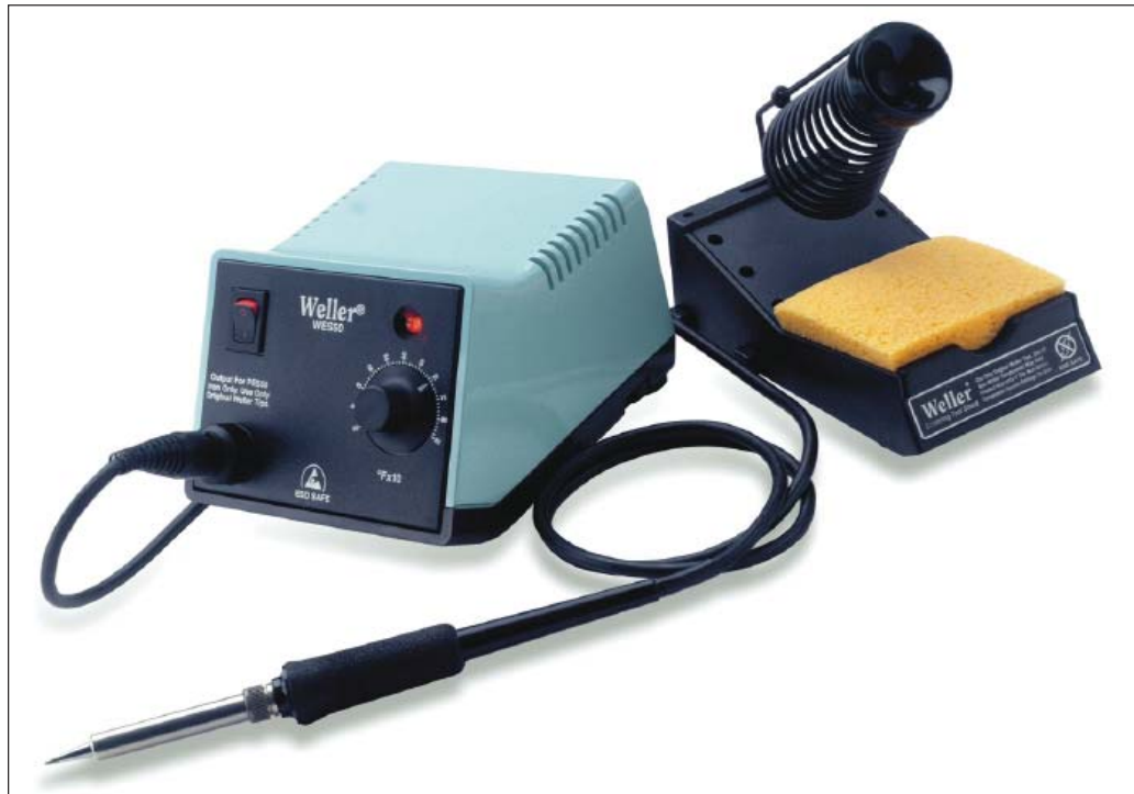
Figure 9-1: Some soldering iron models are temperature-adjustable and come with their own stands.
