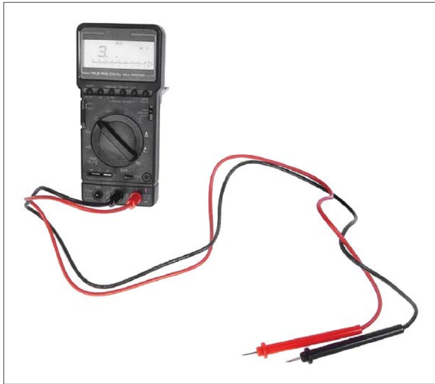
Figure 12-1: Multimeters measure voltage, resistance, current, and continuity.
