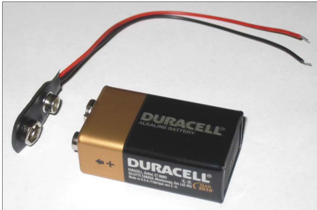
Figure 8-3: A battery clip makes it easy to connect a 9 volt battery to your circuit.
