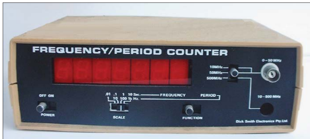
Figure 16-2: A digital frequency counter measures the frequency of a signal.
