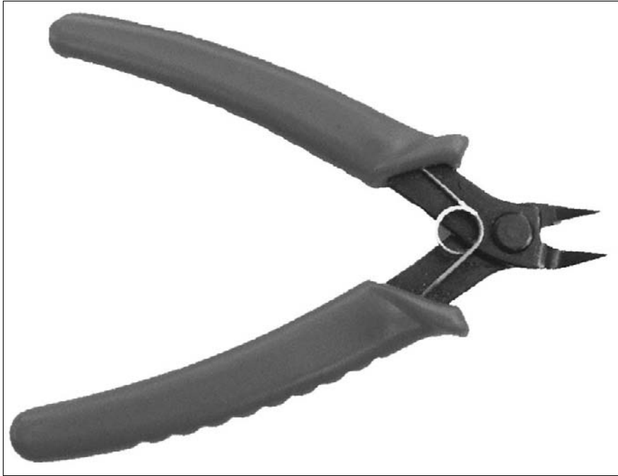
Figure 9-3: Nippy cutters trim wire ends flush to the surface.
