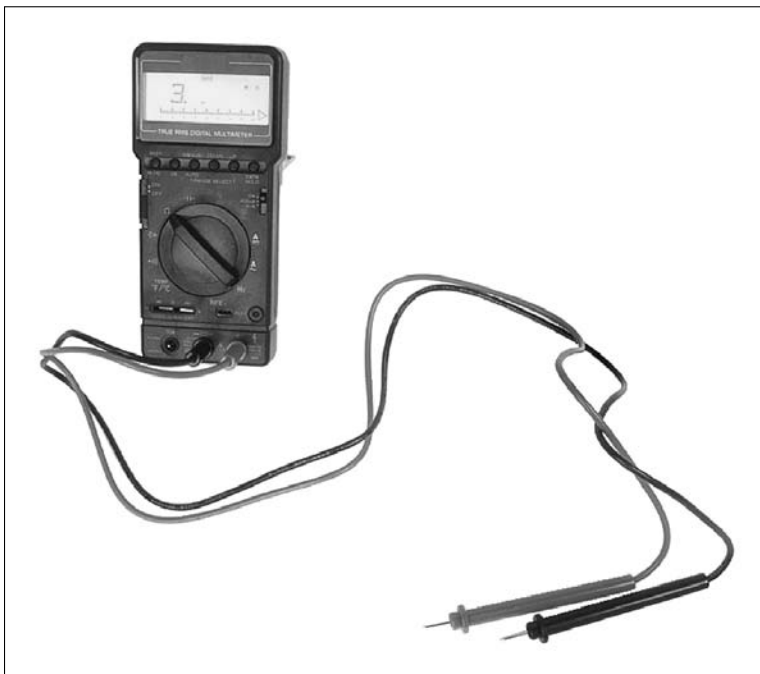
Figure 12-1: Multimeters measure voltage, resistance, current and continuity.
