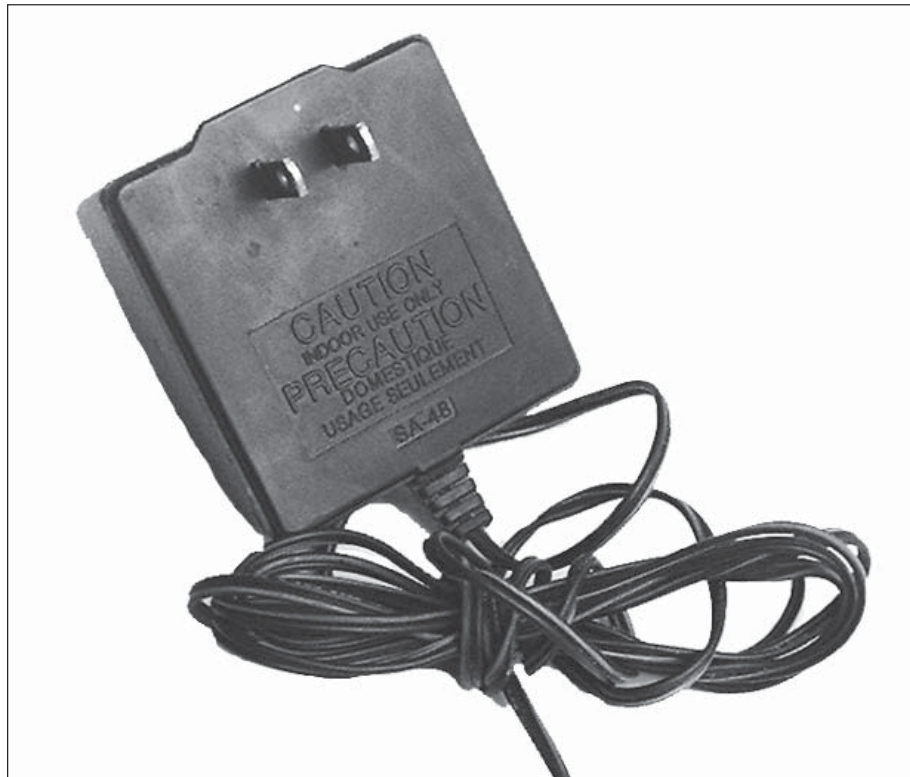
Figure 2-2: A plug-in wall transformer shields you from exposed AC household current.
