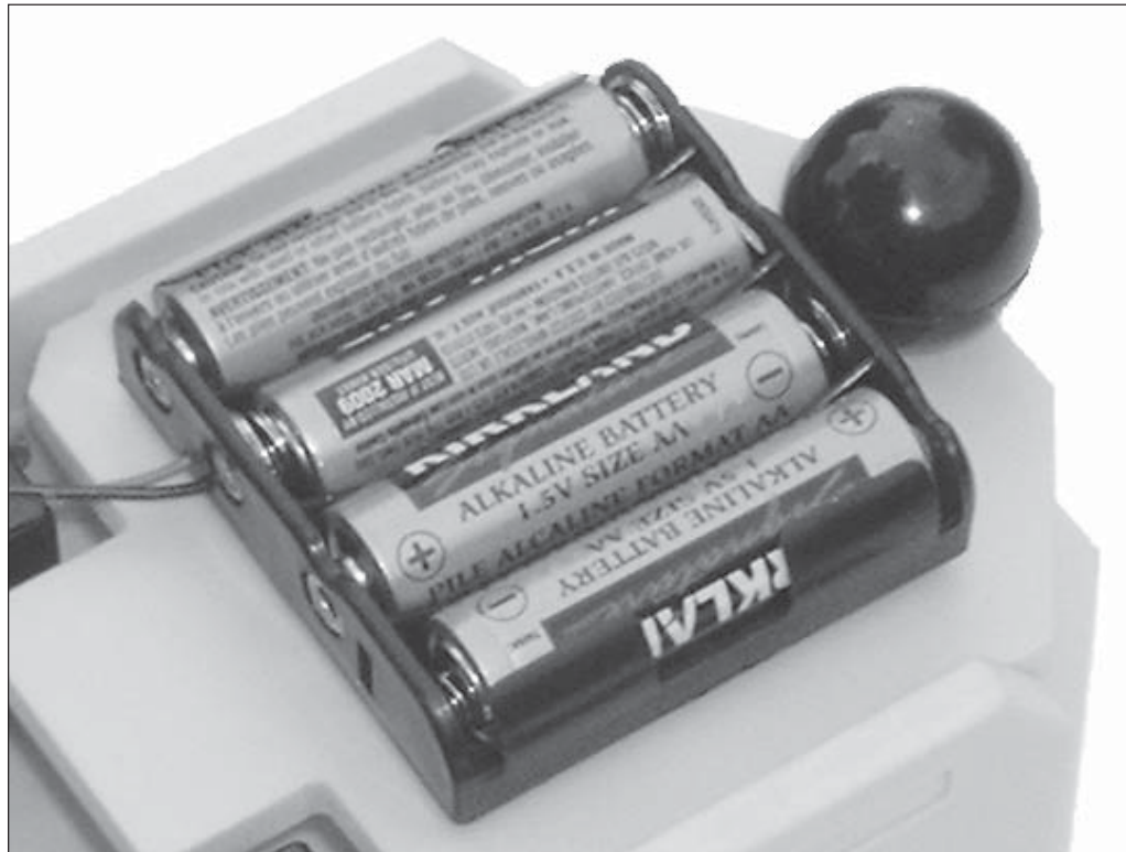
Figure 5-5: Four 1.5-volt batteries tucked into a battery holder produce about 6 volts.
