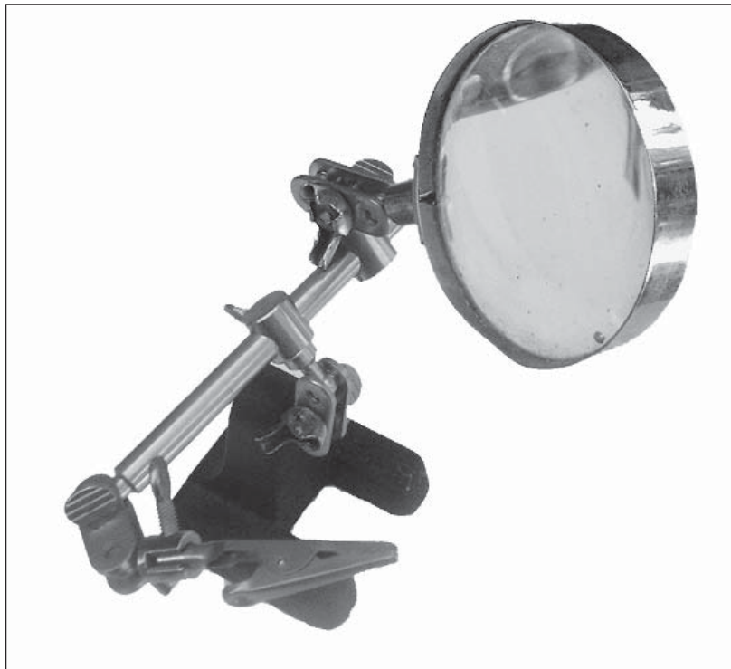
Figure 3-4: These helping hands combine alligator clips with a magnifying glass.
