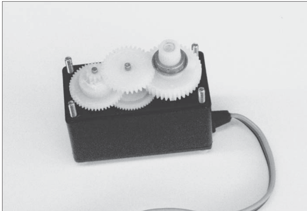
Figure 15-13: A taken-apart servo. Note the placement for all the gears.
