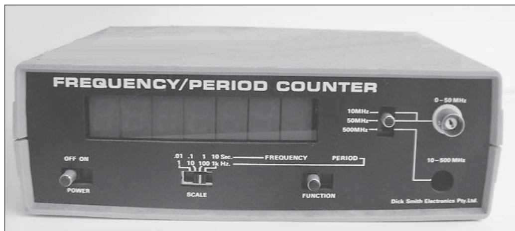
Figure 16-2: A digital frequency counter adds up frequencies.
