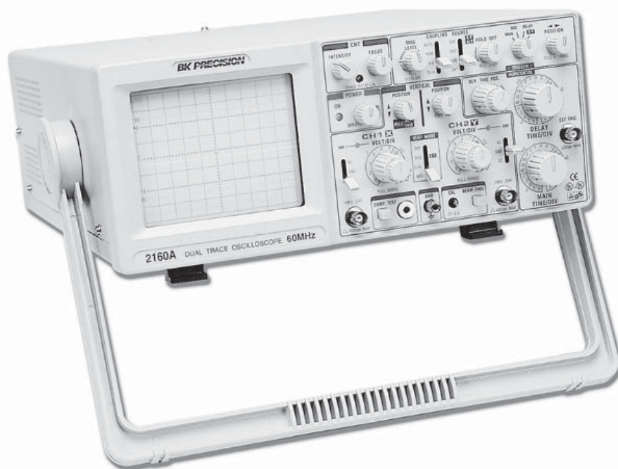
Figure 10-7: A bench scope sits on your worktable and is completely self-contained.
