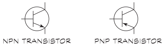
Figure 4-12: Schematic symbols for NPN and PNP transistor types. For an NPN, the arrow points out from the center of the symbol. For a PNP, the arrow points in.
