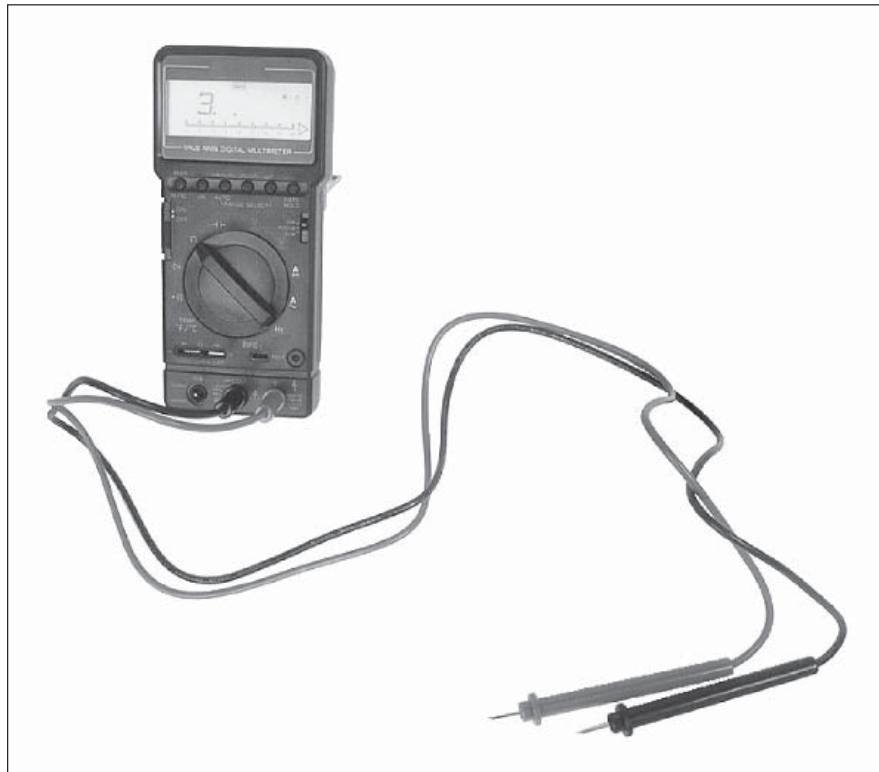
Figure 9-7: On automatic ranging multimeters, setting the desired test function automatically selects the range.
