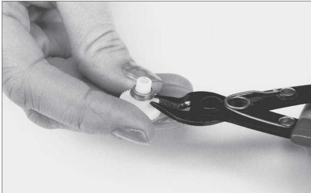
Figure 15-15: Clipping off the ridge on the top of the output gear. Use caution!
