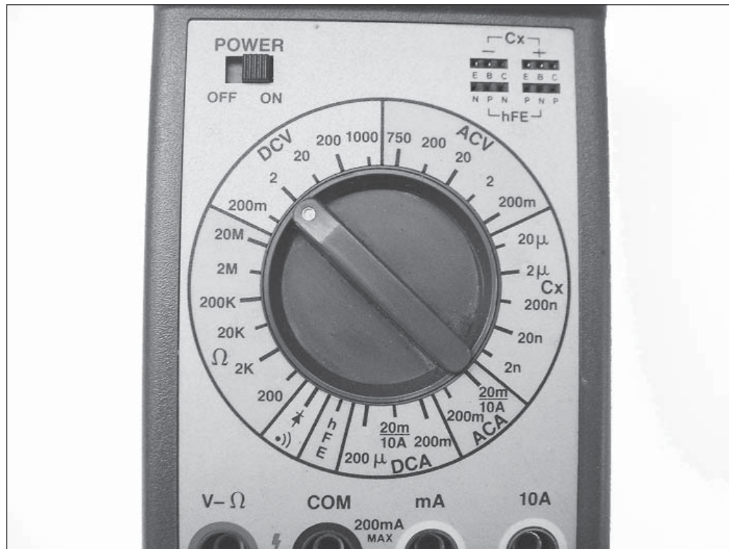
Figure 9-6: Dial in the proper range before taking a measurement when using a multimeter without an automatic ranging feature.
