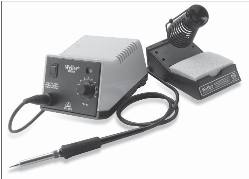
Figure 8-1: Some soldering pencil models are temperature-adjustable, and come with their own stand.
