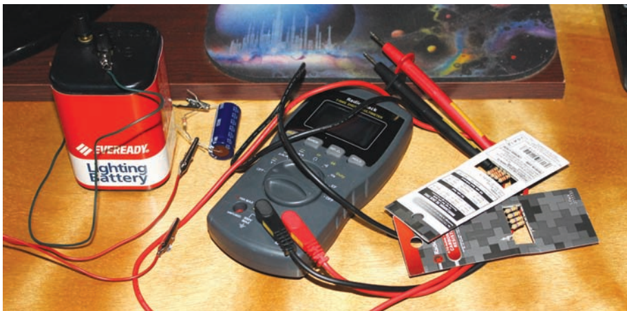
FIGURE 3-10 Components for the discharge experiment include a 6-V battery, a multimeter, two clip leads, a 2200-μF 50-V capacitor, a 3.3k resistor, and a 47k resistor. (Radio Shack sells resistors in packs of five.)
