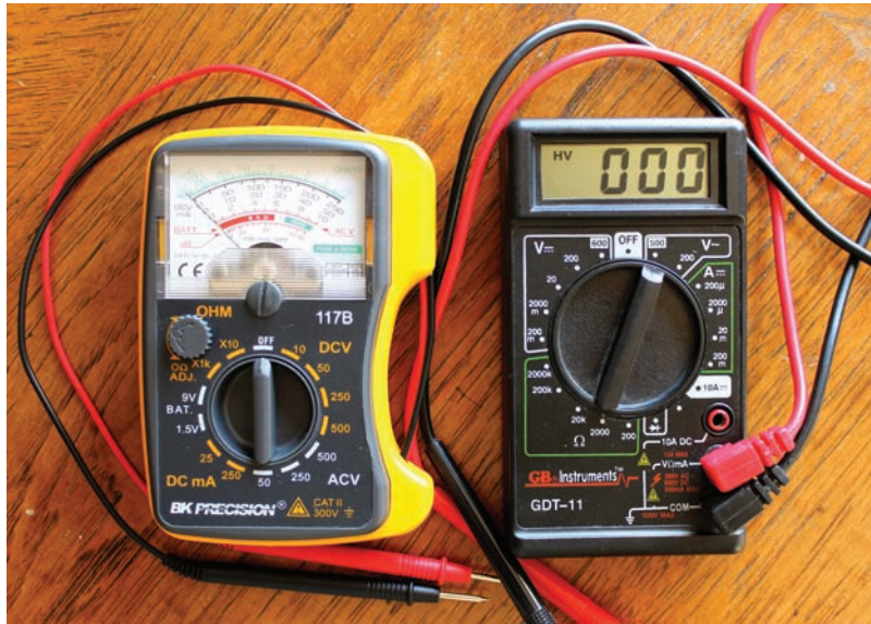
FIGURE 1-4 At left, an analog multimeter. At right, a digital multimeter.
