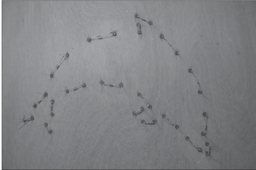
Figure 10-17: Resistors soldered and leads clipped.
