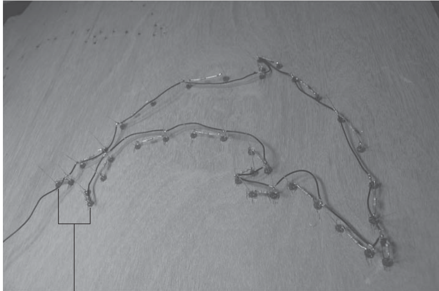
Figure 10-18: Black wires connecting short leads of LEDs.
