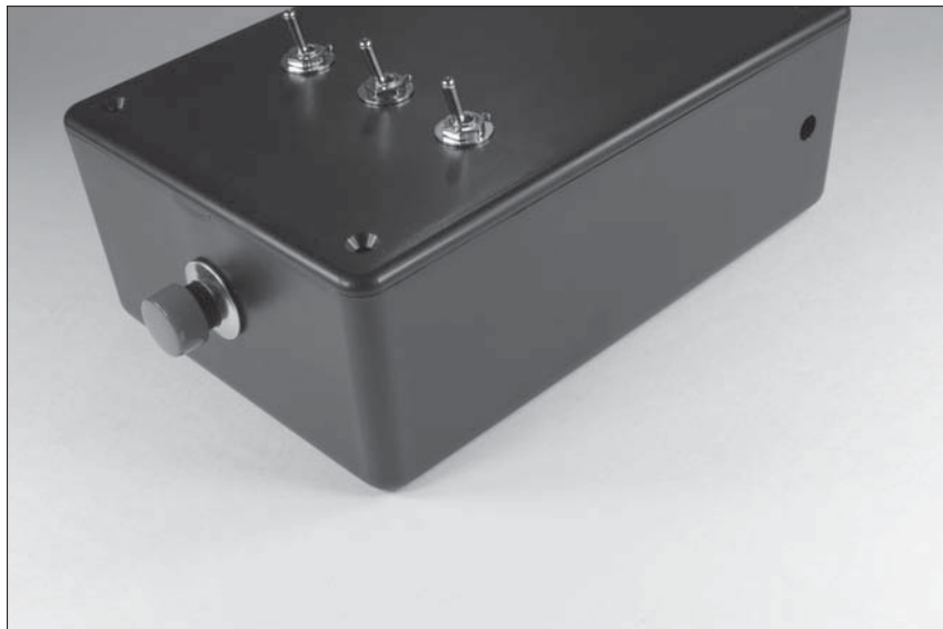
Figure 13-14: Use this hole to feed the antenna out of the box.
