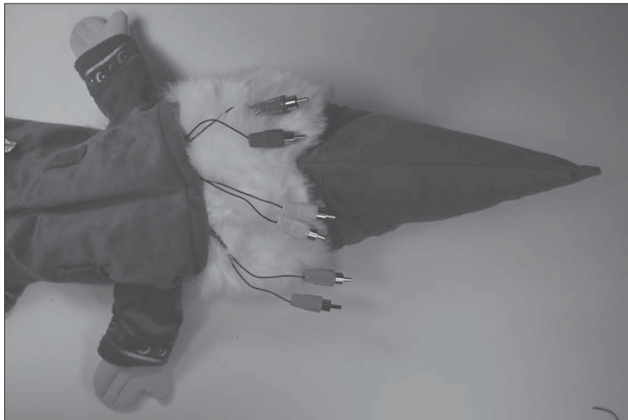
Figure 7-18: Place tactile switches in the puppet.
