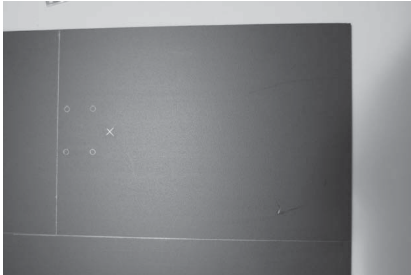
Figure 11-34: Mark the base for cutting and drilling.
