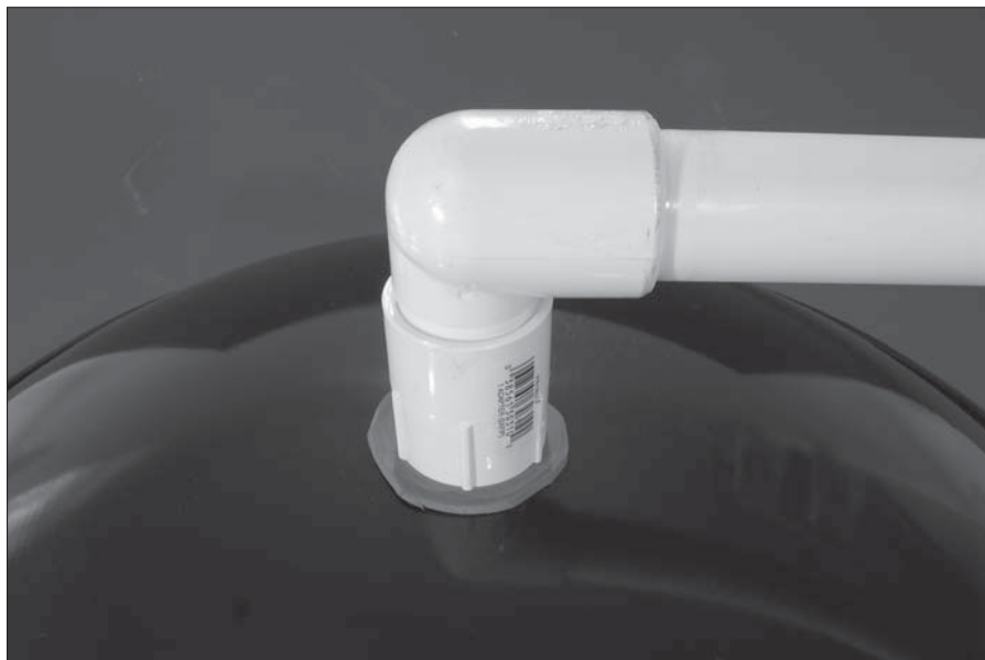
Figure 6-11: Fittings assembled on the parabolic dish.
