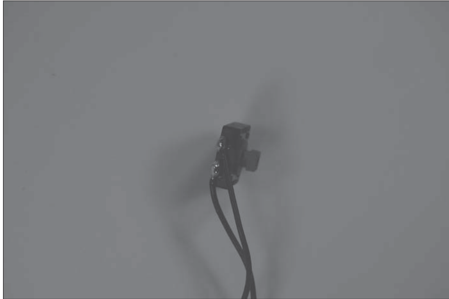
Figure 7-16: Solder wires to tactile switches.
