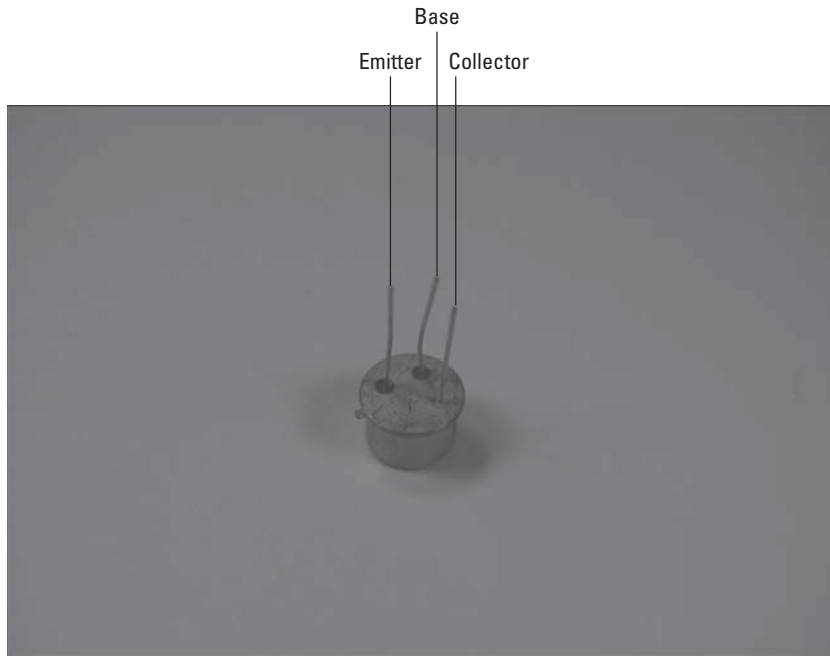
Figure 10-9: The 2N3053 transistor pinout.
