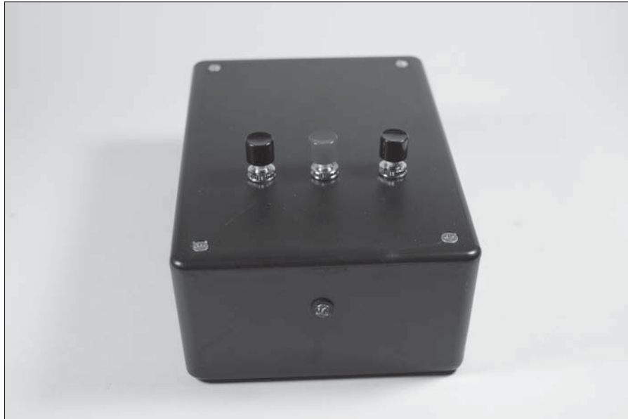
Figure 11-22: The transmitter all put together.
