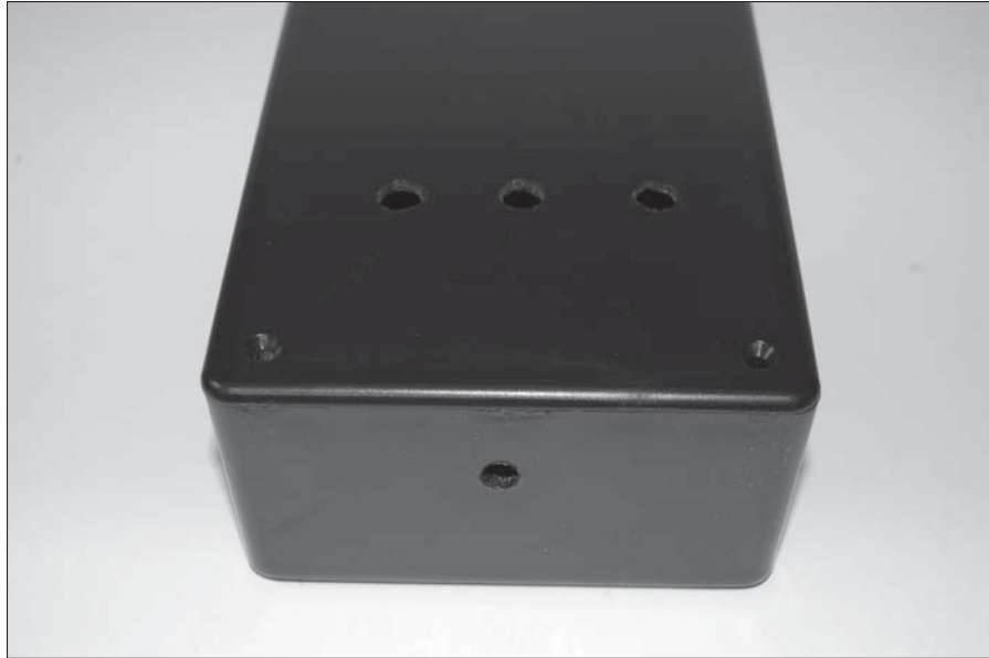
Figure 11-14: Drill holes for the LED and switches.
