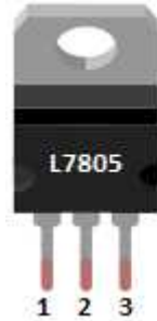
Figure 7-16: Typical 78xx voltage regulator with pin configuration
