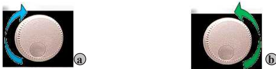
Figure 5-35: Turn the knob in clockwise (a) to increase frequency, Turn the knob in anticlockwise (b) to decrease the frequency
