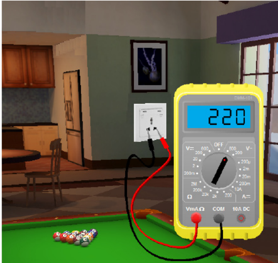
Figure 4-4: Test electrical wall outlet using voltmeter
