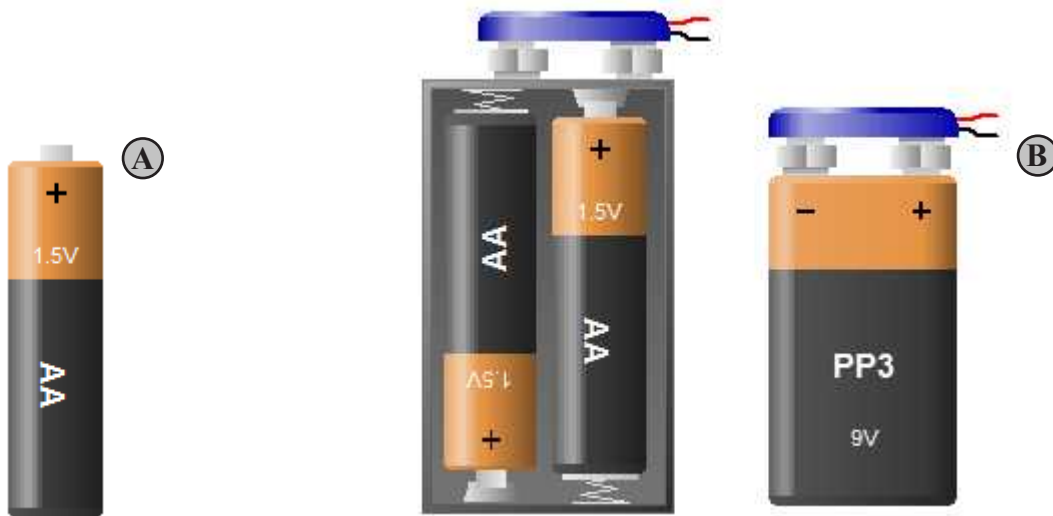
Figure 3-12: Size of common batteries. AA Cell (A) and Batteries DC source (B)
