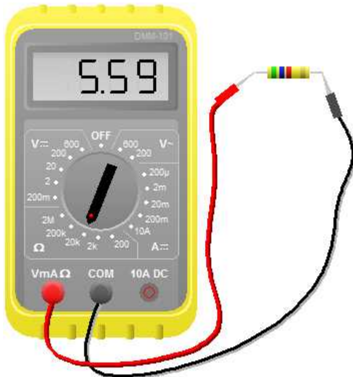
Figure 5-2: Multimeter set in Ohm's range to measure resistance
