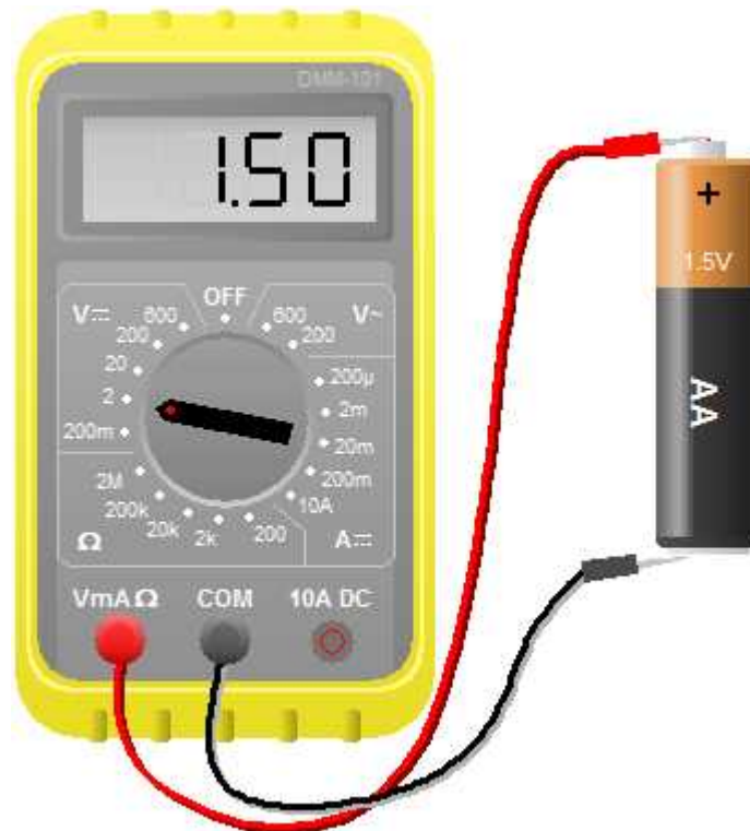
Figure 4-5: Measuring Voltage of an AA cell battery
