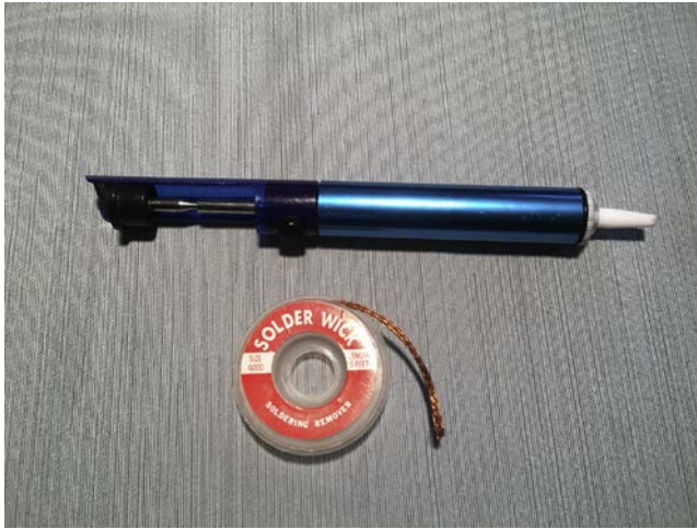
FIGURE 14.6 Tools for desoldering, a solder sucker and solder wick.
