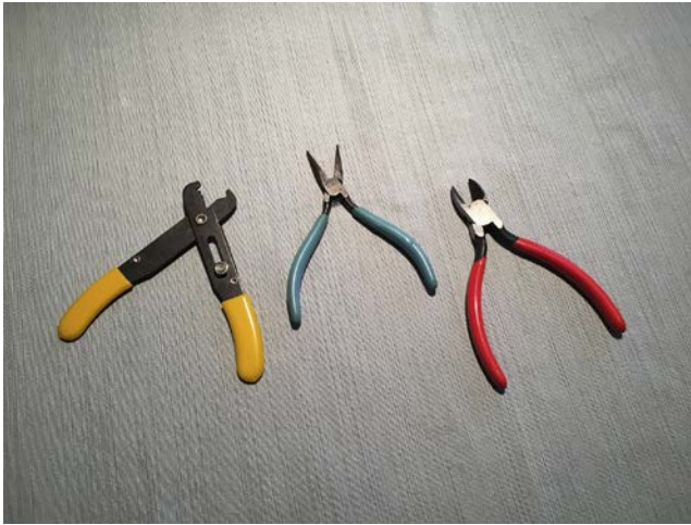
FIGURE 14.2 Tools used in soldering. On the left is a wire stripper. Next is a pair of needle-nose pliers. On the right is a side cutter for wire.
