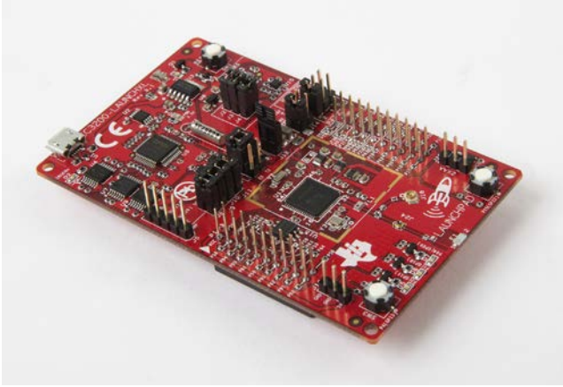
FIGURE 13.12 The Texas Instruments' LaunchPad development board uses an MPS430 microcontroller.
