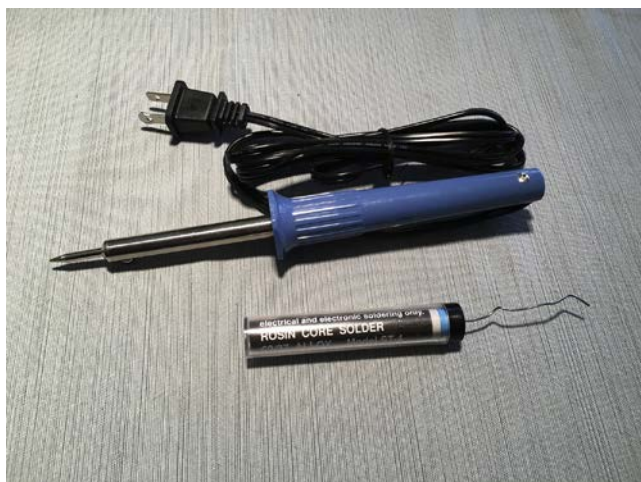
FIGURE 14.1 A common soldering iron used in electronic work.
