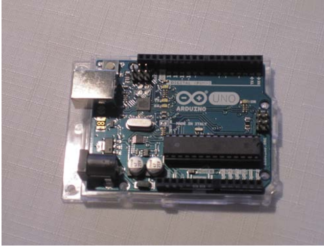
FIGURE 13.11 The Arduino Uno R3 is one of the most widely used microcontroller learning platforms.
