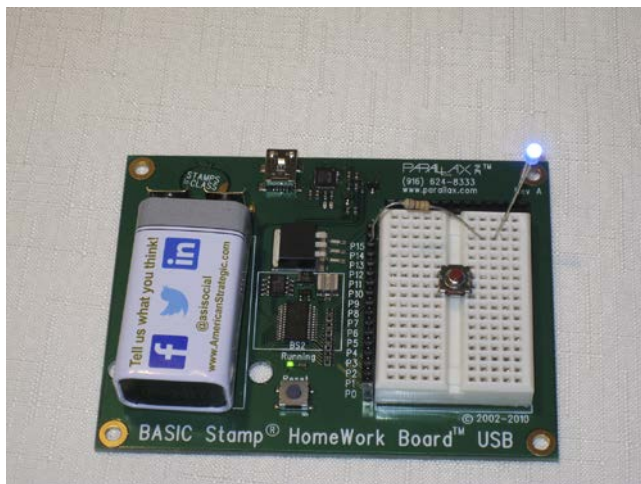
FIGURE 13.10 The Parallax BASIC Stamp Activity Kit experimental board is designed to be operated from a 9-V battery. The PIC MCU is the IC above the reset button in the center.
