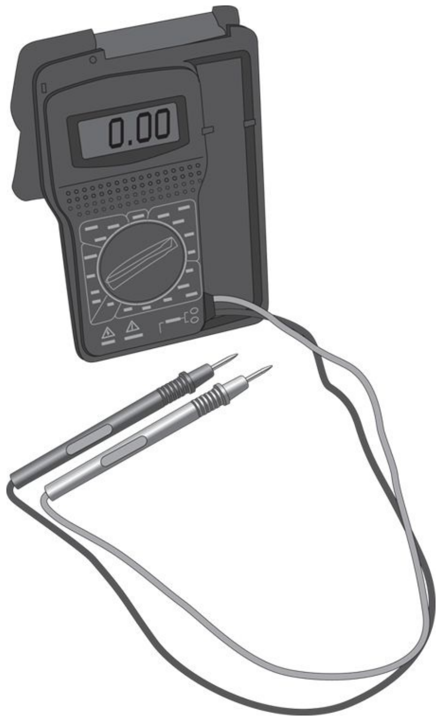
FIGURE 2-3: You can use a multimeter like this to measure voltage.
