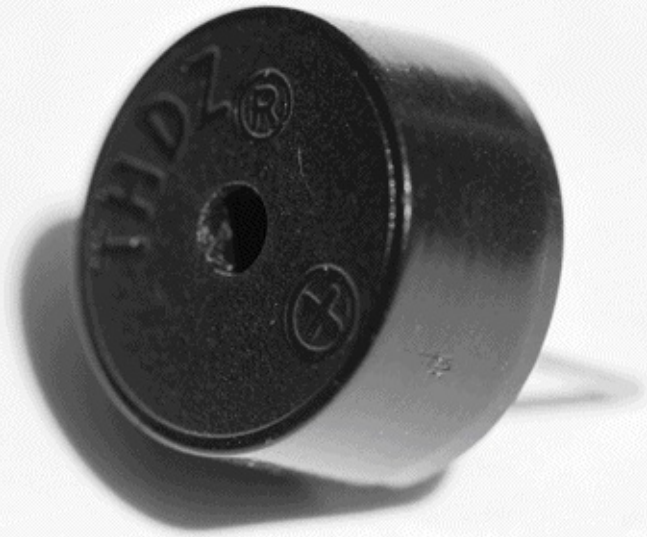
FIGURE 4-1: The piezoelectric speaker that comes with the BASIC Stamp Activity Kit.
