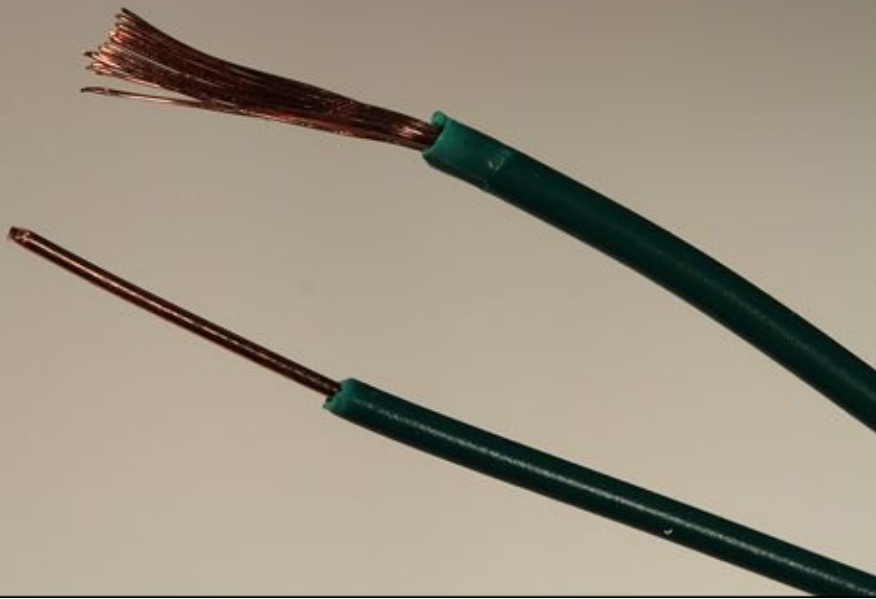
FIGURE 3-11: Solid and stranded wire.
