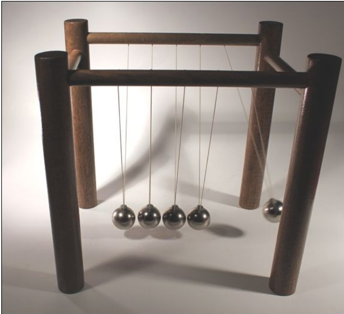
FIGURE 2-4: Newton's Cradle works much like alternating current.
