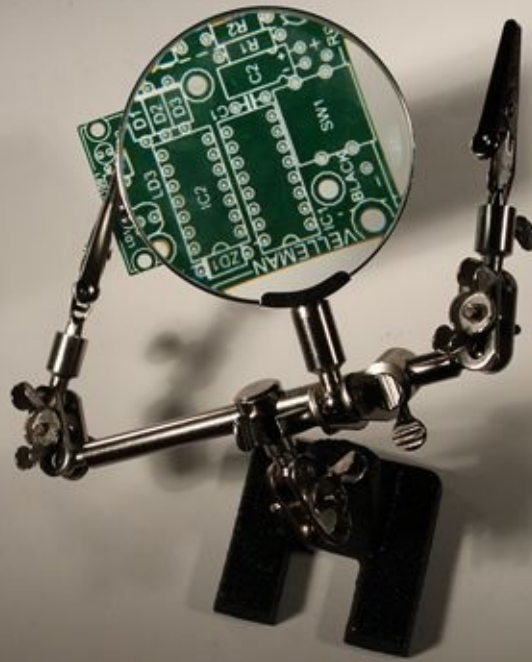
FIGURE 3-6: A third hand can hold your stuff so both your hands are free to do the work.
