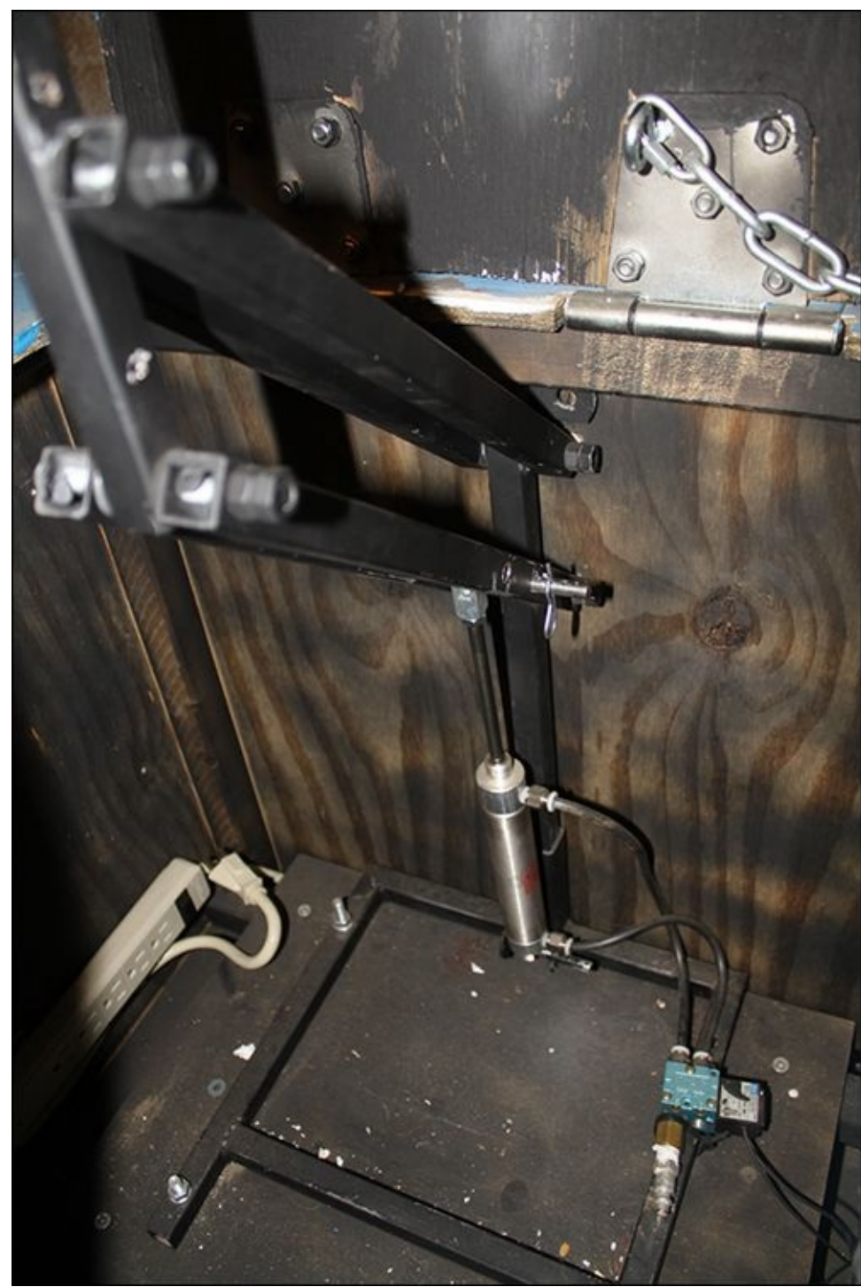
FIGURE 3-2: The lift mechanism.
