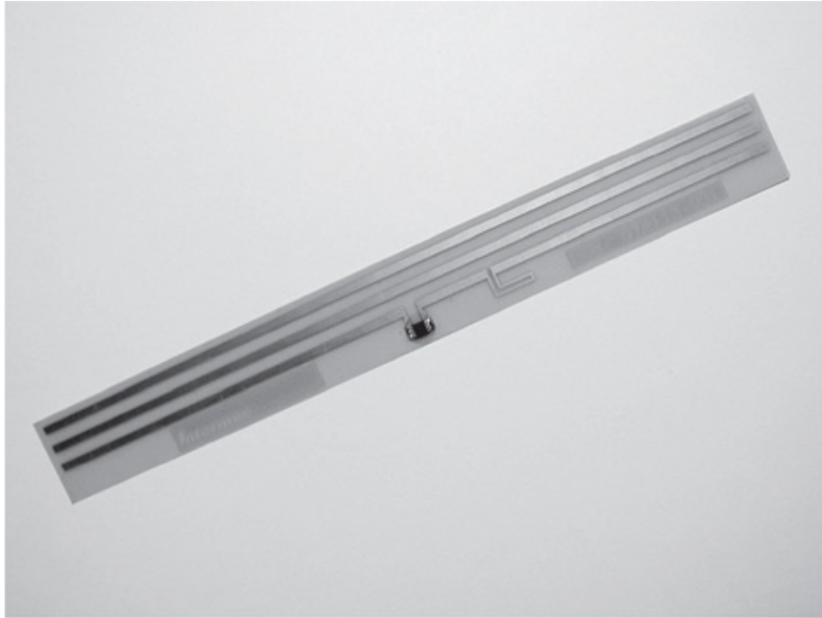
FIGURE 2.4 Typical passive radio frequency–identification (RFID) tag showing the antenna made from copper. (Courtesy of Pavel Nikitin, Intermec Technologies Corporation, Everett, WA.)
