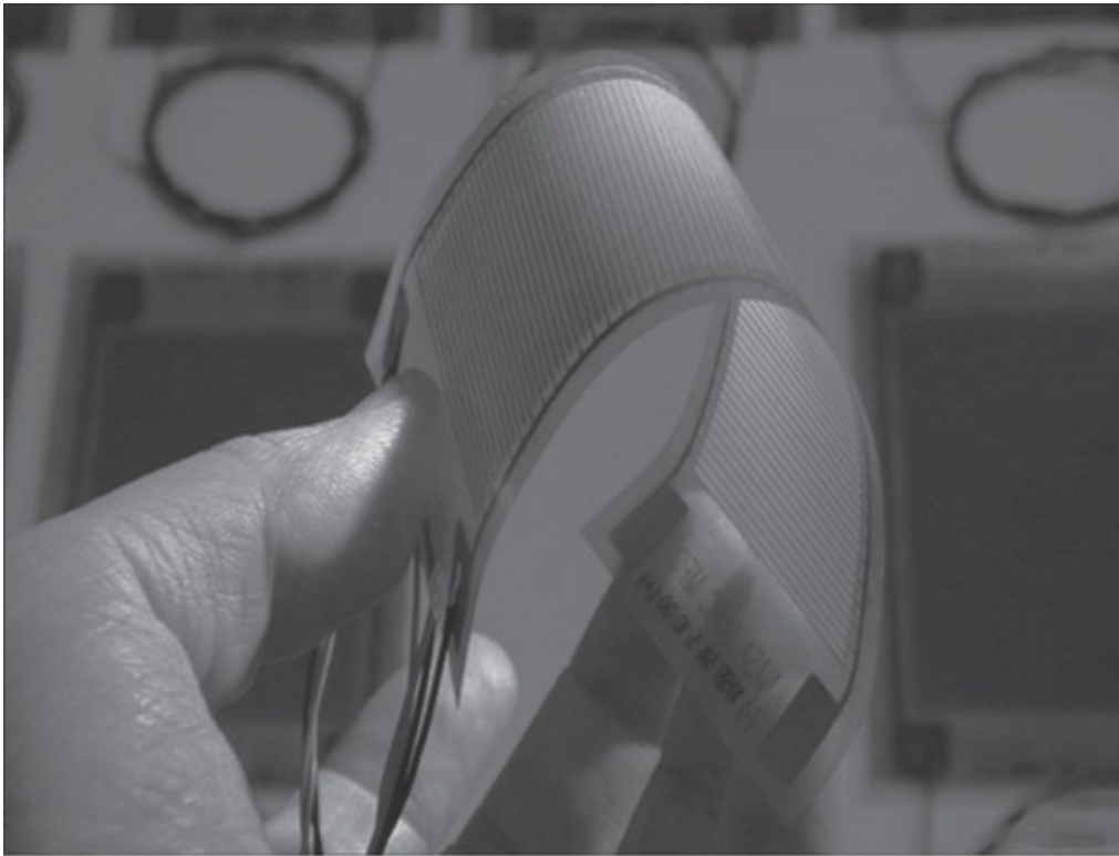
FIGURE 10.42 Photograph of a zirconium titanate (PZT)-based flexible macro fiber composite. (Courtesy of Smart Material Corporation, Sarasota, Florida.)
