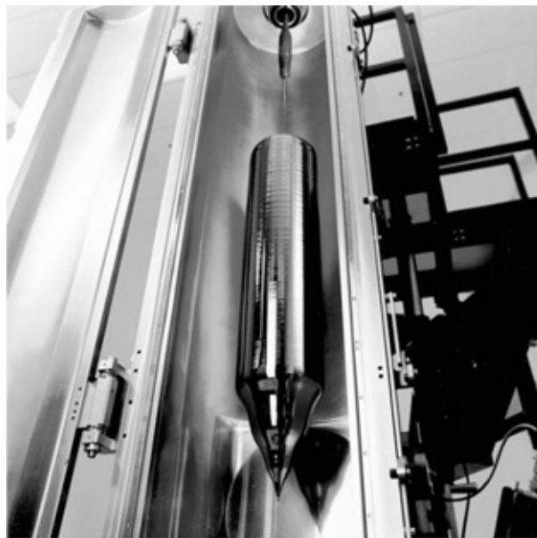
FIGURE 1.5 Single crystal of silicon. (From Askeland, D. and Fulay, P., The Science and Engineering of Materials , Thomson, Washington, DC, 2006. With permission.)
