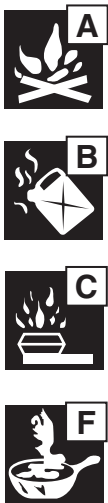
Figure 25.1 Standard pictograms for use on fire extinguishers illustrating the types of fire they can be used on.
