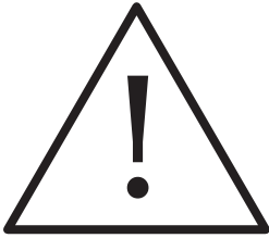
Figure 19.5 Components marked with this symbol in the service schematic are safety critical and should be replaced with identical types, as directed by the service manual
