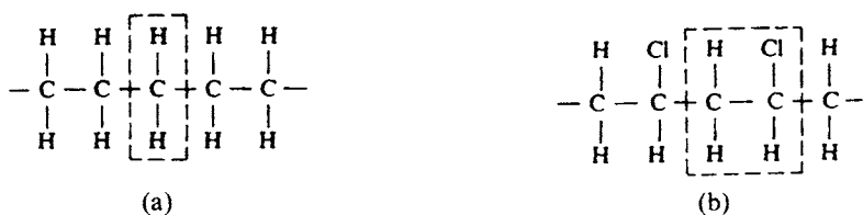
Figure 9.1. (a) Polyethylene. (b) Polyvinylchloride. (The dashed enclosures mark the repeat unit. Polyethylene is frequently depicted as two \text{CH}_2 repeat units for historical reasons.
