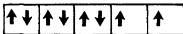
Figure 15.4. Schematic representation of the spin alignment in a d -band which is partially filled with eight electrons (Hund's rule).
