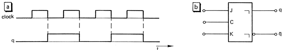
Figure 19.13. (a) A JK flip-flop can act as a digital frequency divider for jk = 11 : the output frequency is half the clock frequency, (b) the circuit symbol of a master-slave JK flip-flop.
