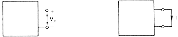
Figure 5.1. The determination of the open voltage and the short-circuit current of an active two-terminal network.
