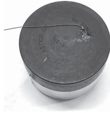
Figure 11-9 Secondary coil bottom.
