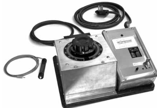
Figure 9-9 Remote switch, variac, and contactor box.
