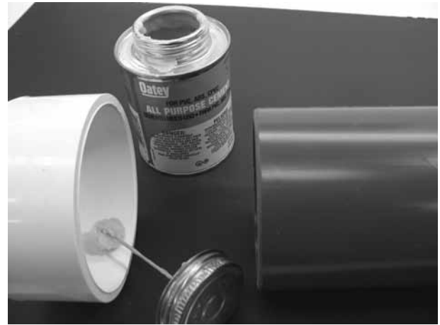
Figure 14-39 Sealing end caps to the enclosure tube.
