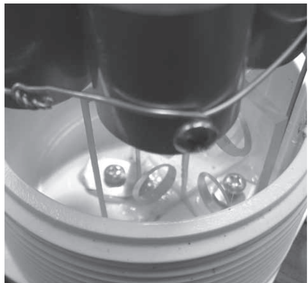
Figure 14-27 Method used for sealing mounting screws.
