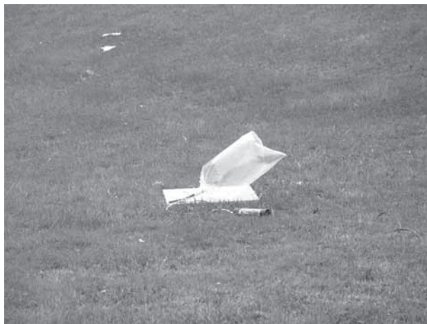
Figure 17-9 Bag filled with HHO gas and attached to remote igniter.
