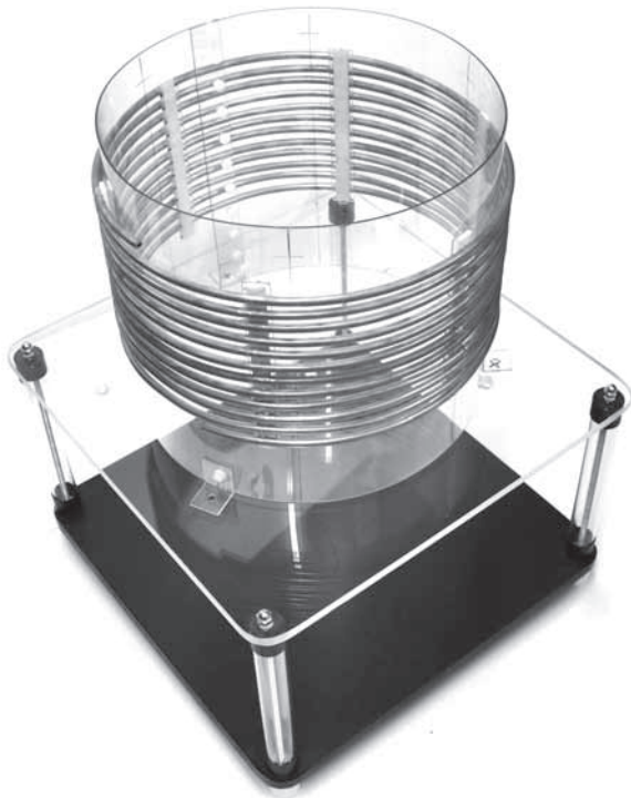
Figure 10-68 Base and primary coil (without strike ring).
