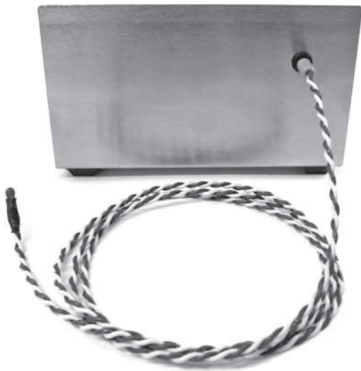
Figure 13-15 Rear-panel with temperature sensor attached.
