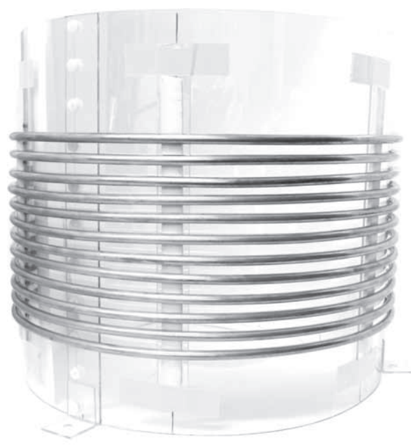
Figure 10-66 Coil spacing around cylinder.
