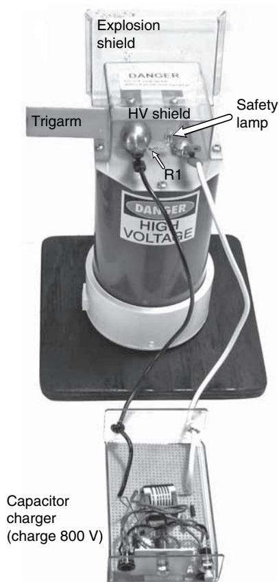
Figure 4-1 Assembled capacitor exploder with charger.
