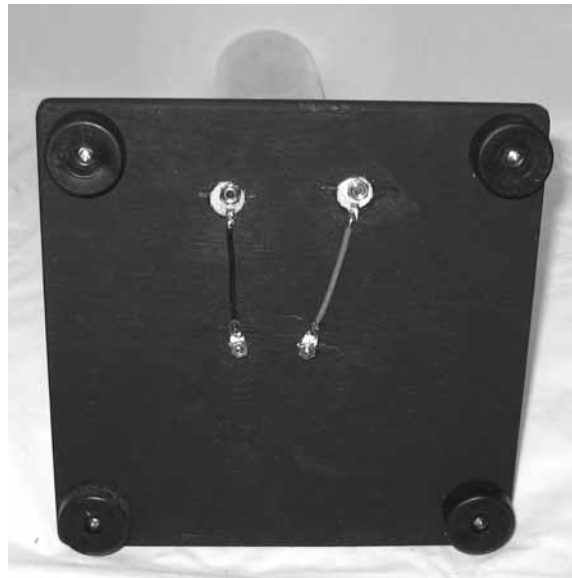
Figure 14-29 Wiring banana jacks to the wooden base.
