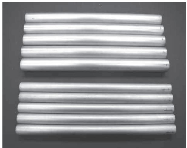
Figure 14-9 Mark for drilling \frac{3}{32} -inch holes.
