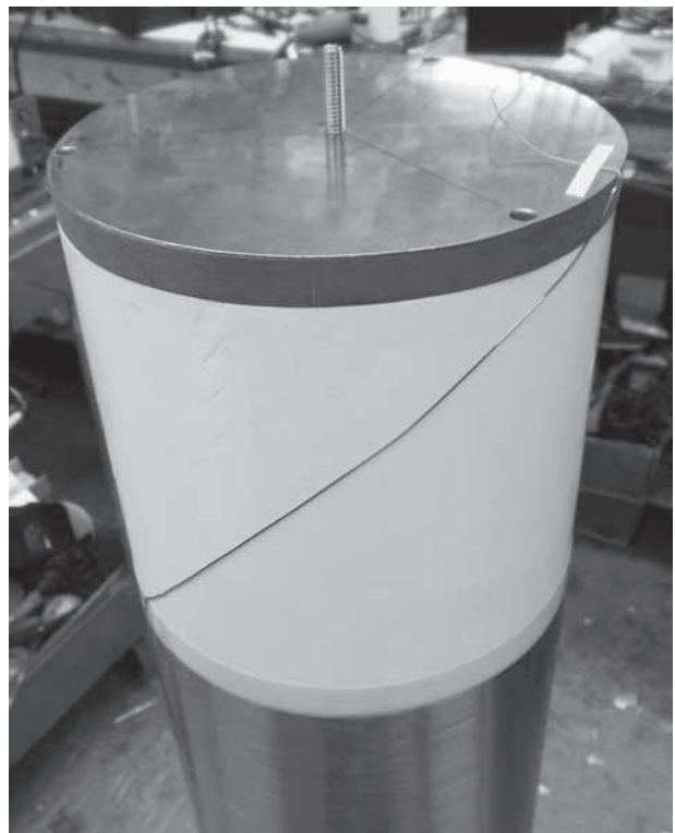
Figure 10-92 Magnetic wire running to top cap.
