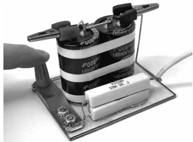
Figure 4-18 Discharging the test jig.
