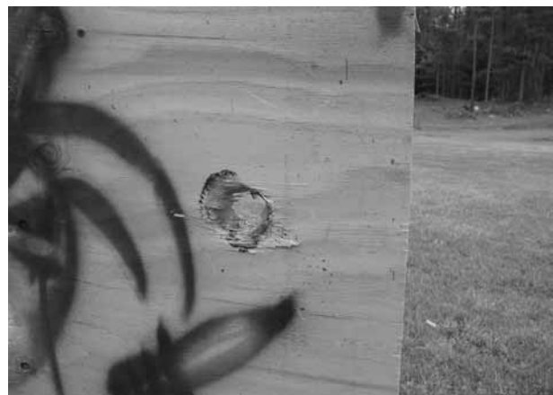
Figure 19-12 Impact of the 50-millimeter projectile from 100 ft.
