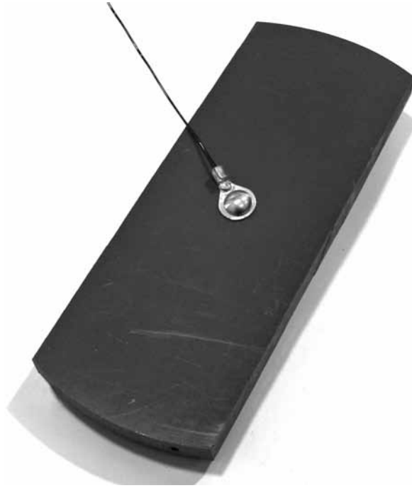
Figure 9-41 Magnetic wire soldered to a terminal attached to a bracket.
