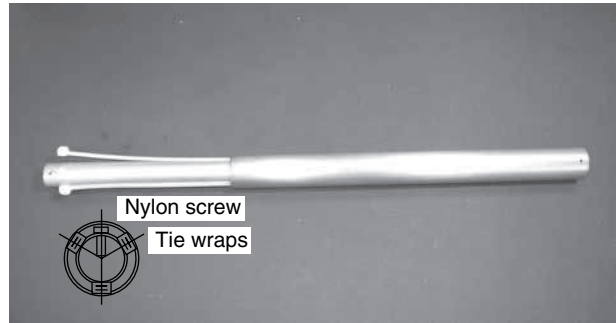
Figure 14-12 Tie wrap spacer placement.
