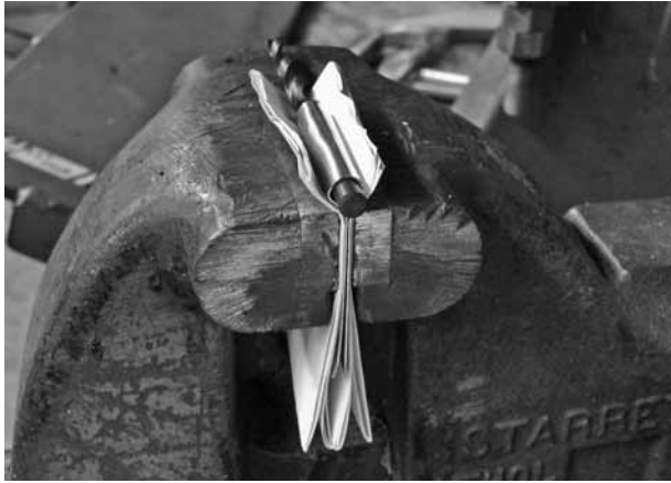
Figure 9-65 Forming the adjusting tap in a vice.
