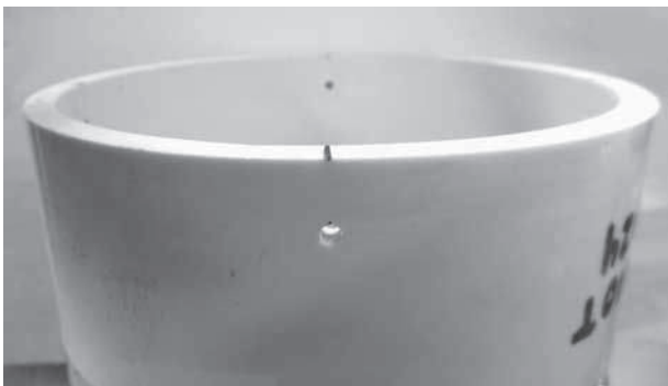
Figure 10-82 Bottom cap securing holes
