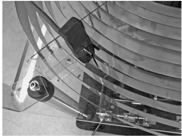
Figure 9-68 Adjusting tap on the primary coil.
