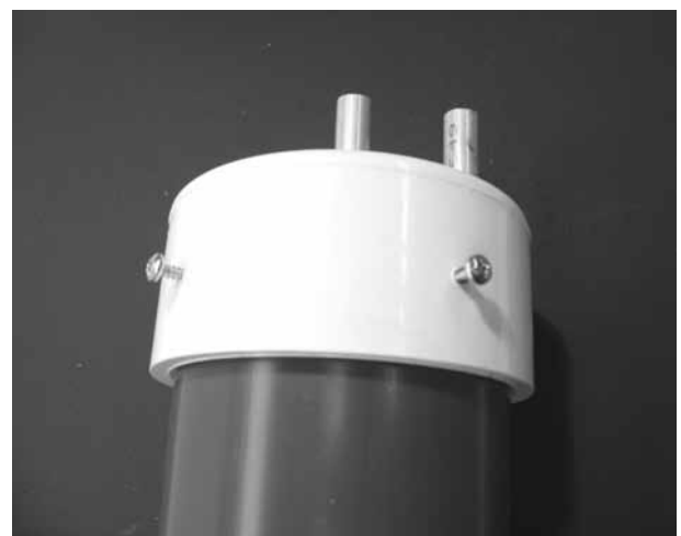
Figure 14-40 Sealing end caps to the enclosure tube with additional screws.
