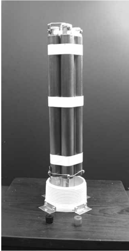
Figure 14-30 Reactor core assembly ready for enclosing into vessel.
