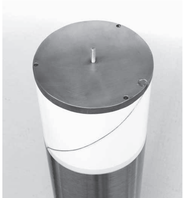
Figure 10-94 Finished top of secondary coil.
