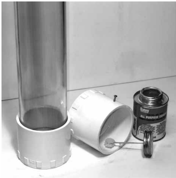
Figure 14-31 Main housing and slip caps.
