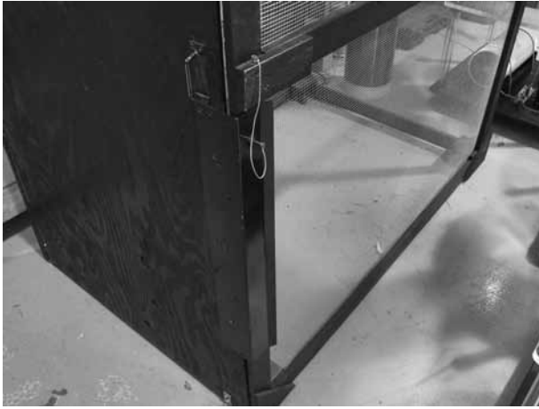
Figure 20-17 A long L-bracket secures the door to the frame.
