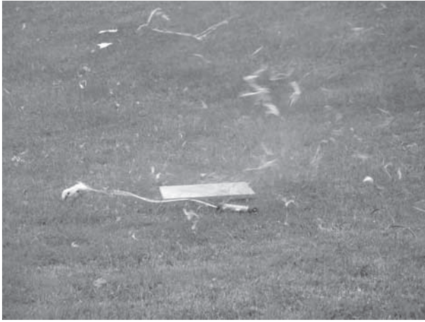
Figure 17-10 Ignition of HHO gas.
