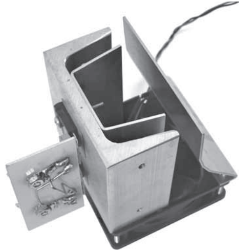
Figure 13-9 FET board attached to heat sink.
