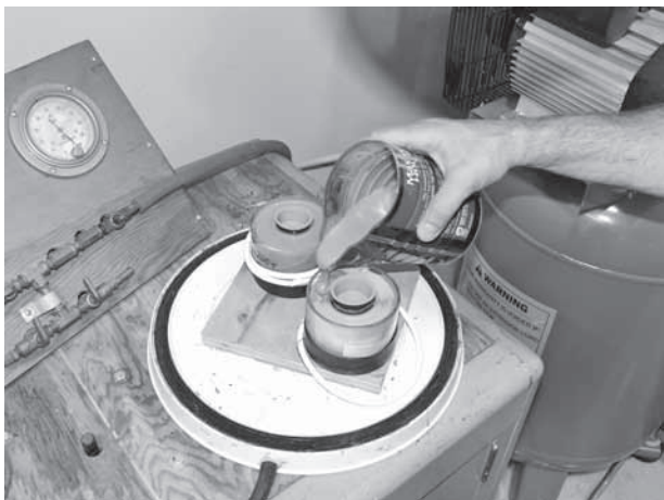
Figure 11-11 Pouring the two-part silicone elastomer goop.
