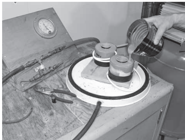
Figure 11-13 More goop in the partially filled coils.
