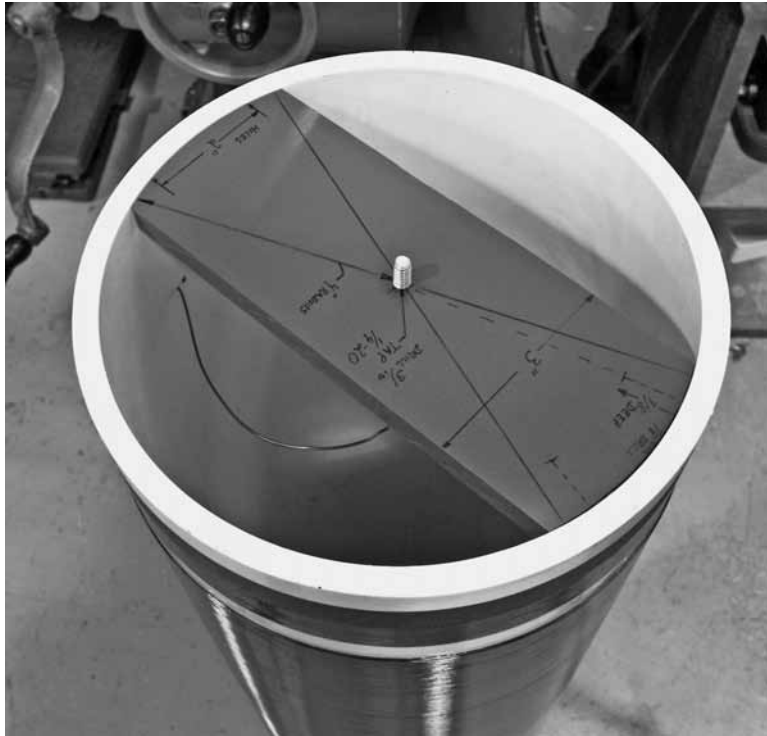
Figure 9-42 End brackets and magnetic wire.
