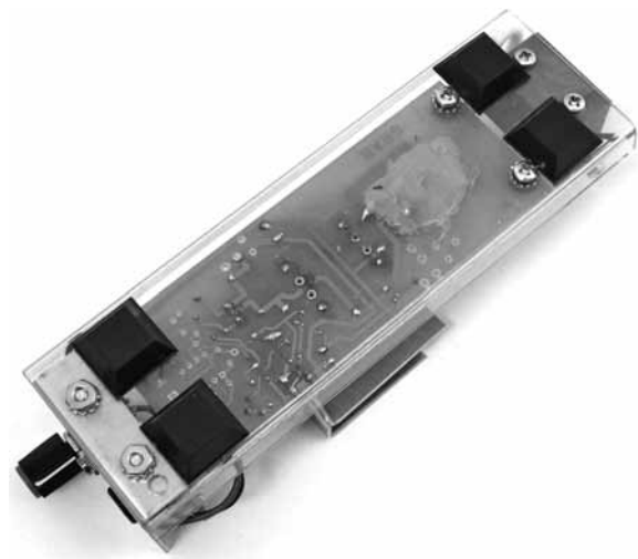
Figure 8-15 Chassis bottom showing securing screws.
