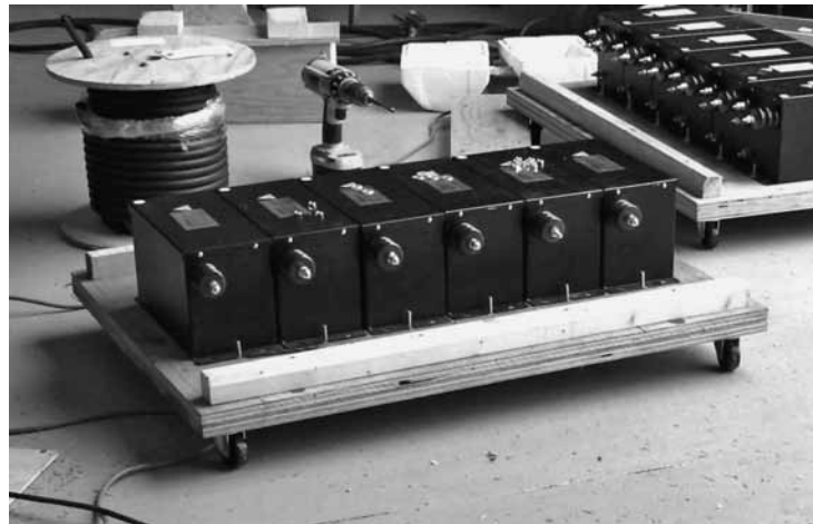
Figure 9-19 Transformers mounted to power supply base.
