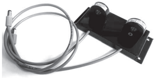
Figure 10-73 Assembled current transformer bracket.
