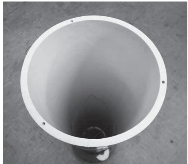
Figure 10-80 Holes drilled into top end of PVC tube.
