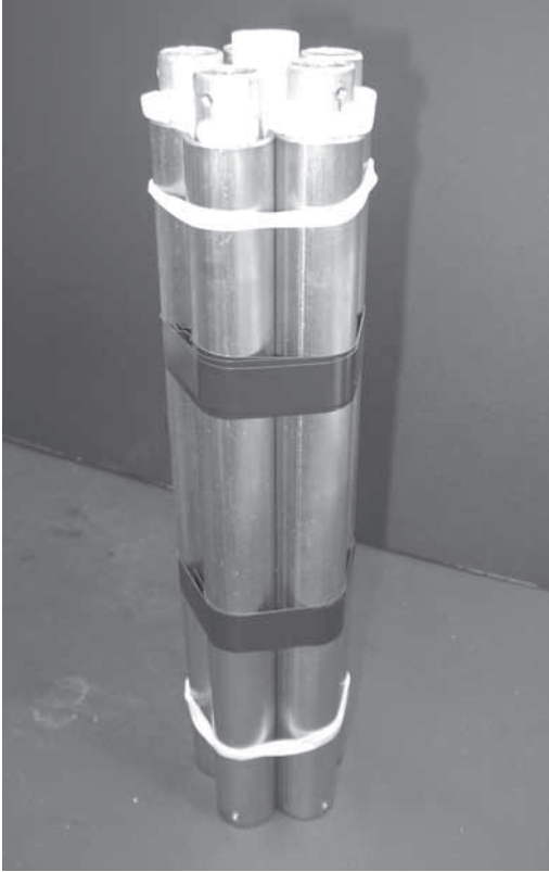
Figure 14-18 Tube assembly showing method of attaching together.
