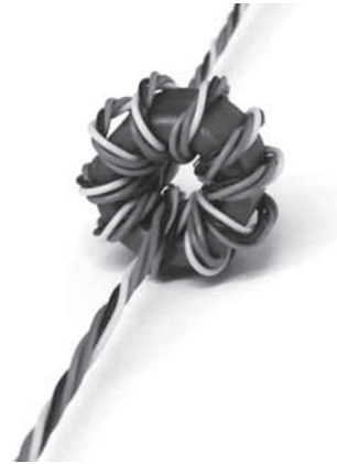
Figure 10-18 Equidistant spacing of four-strand winding.
