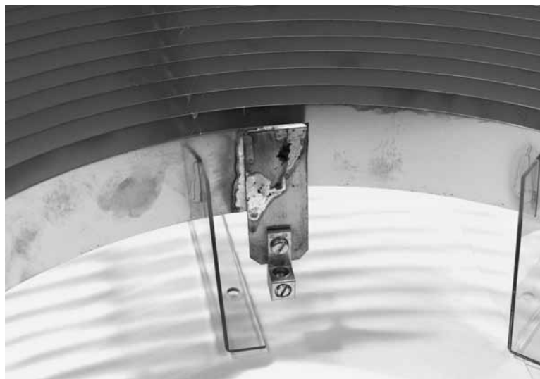
Figure 9-36 Primary coil ribbon attachment with terminal block.
