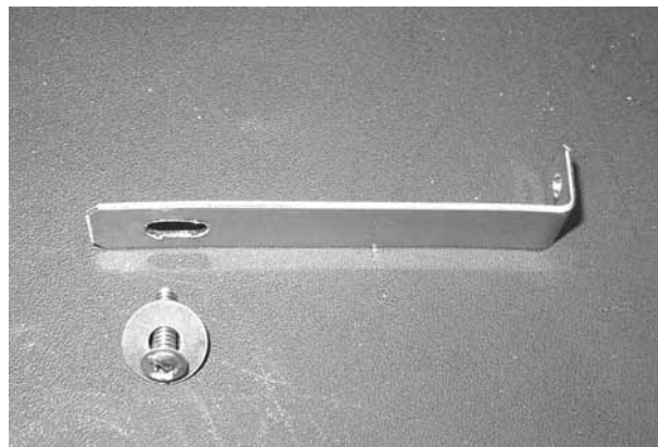
Figure 14-24 Negative electrode fabrication from 3½- x ½- x 1/16-inch stainless.
