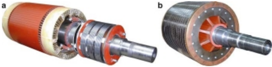
Fig. 9.1 (a) Slip ring rotor and (b) squirrel cage rotor
