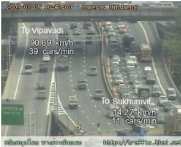
Fig. 21.5 Image classified as jam traffic by ANN and as light traffic by OR technique
