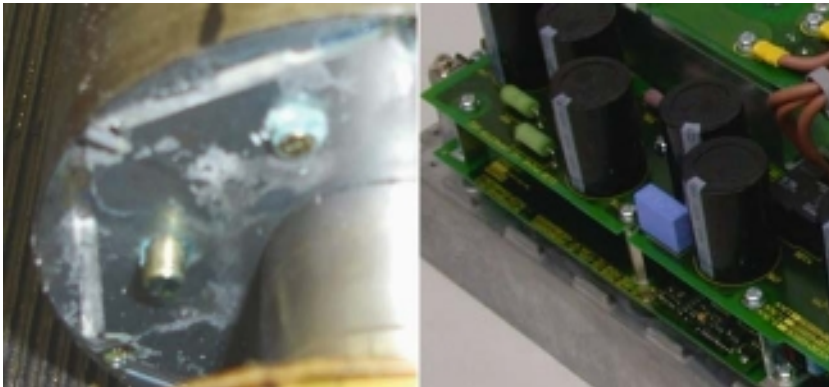
Fig. 3.2 Typical interior permanent magnet machine construction ( left ) and power electronic with DC-link ( right )
