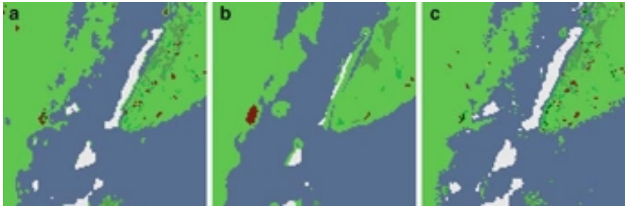
Fig. 40.5 Impact of window size on the pre-classification accuracy. a- Ray_s^2 = 1 , b- Ray_s^2 = 10 , c-auto-adaptative Ray_s
