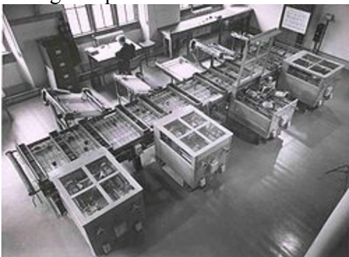
Cambridge differential analyzer, 1938
