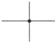
Conductor connection or junction
