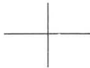
Unconnected crossing conductors
