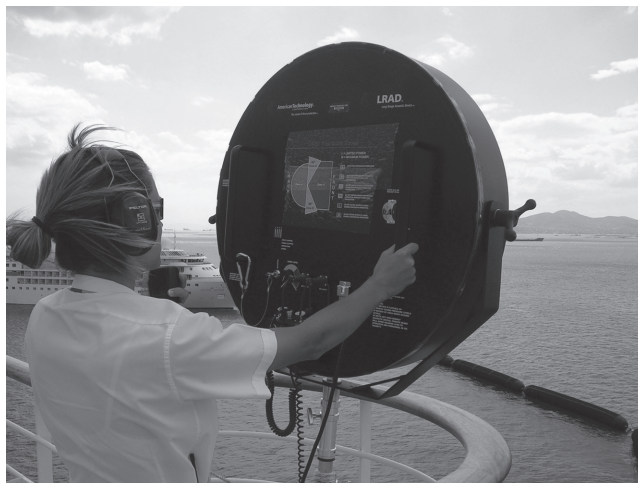
FIG. 6 LRAD (Long Range Acoustic Device) 1000X. (Courtesy of LRAD Corporation.)
