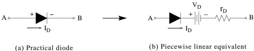
Figure 2.20. Representation of a practical diode by its piecewise linear equivalent
