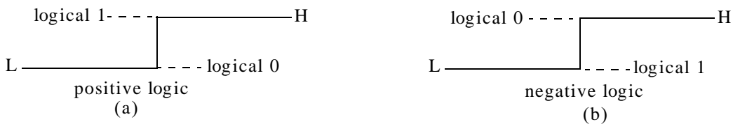
Figure 6.4. Positive and negative logic defined
