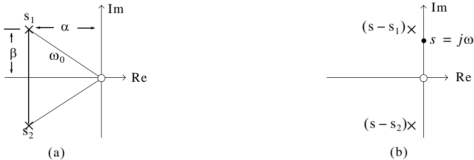
Figure 9.10. Graphical representation of the relations s_1 = -\alpha + j\beta , s_2 = -\alpha - j\beta , and \beta^2 = \alpha^2 - \omega_0^2
