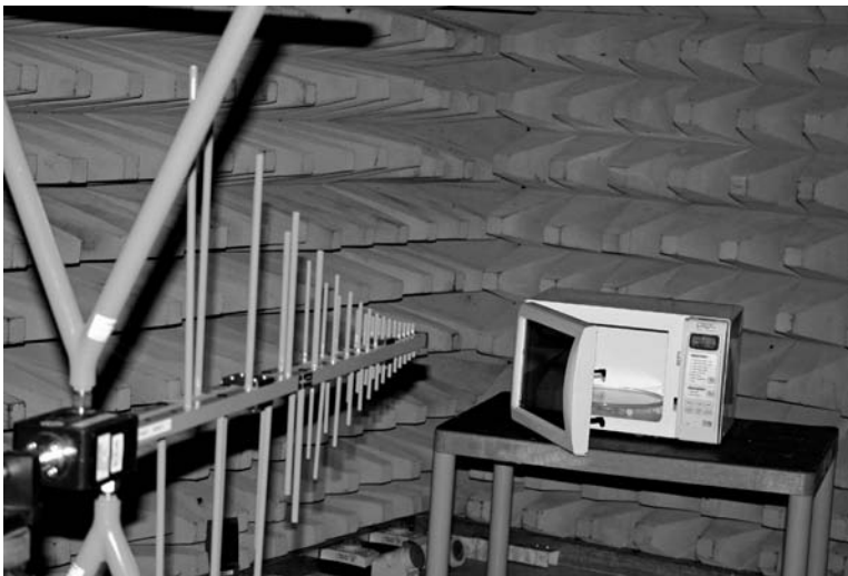
Figure 10.1 A microwave oven under test for electromagnetic emissions in a test chamber lined with cones of radio-absorbing material. (Courtesy of TÜV Product Service Ltd.)
