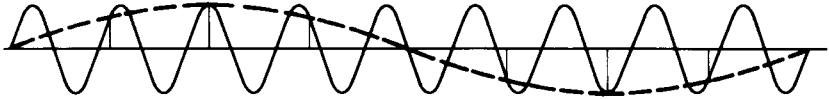
FIGURE 22-2 Fast diodes are switched to obtain samples of a gigahertz wave at successively later points on the cycle. The average of the samples is a low-frequency wave that can be amplified and displayed easily.
