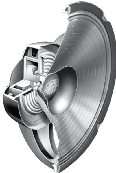
FIGURE 2.2 Loudspeaker incorporating a whizzer cone.
