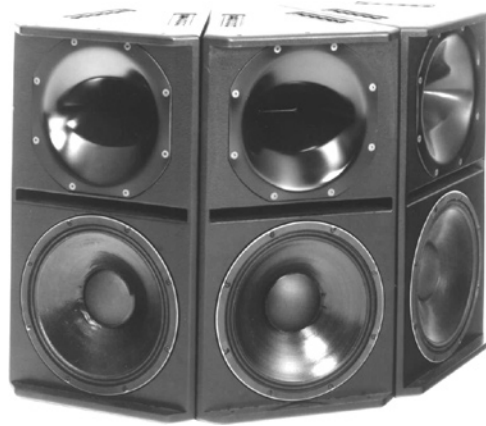
FIGURE 3.12 TRAP arrays can be quite small; however, the size of the horns will determine the lower frequency limit at which the True Array Principle ceases to operate.
