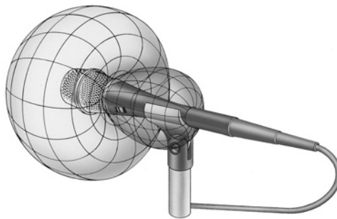
FIGURE 1.8 Supercardioid pickup pattern. Courtesy Shure Incorporated.
