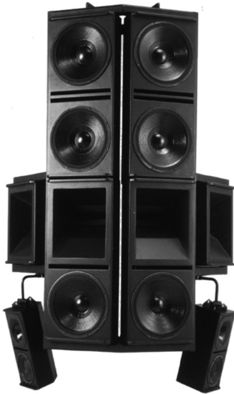
FIGURE 3.13 Reference Point Array using four 40^{\circ} \times 40^{\circ} mid-high enclosures and six low-frequency modules in Tri-Polar configuration for vertical pattern control, along with appropriate small full range systems for downfill.
