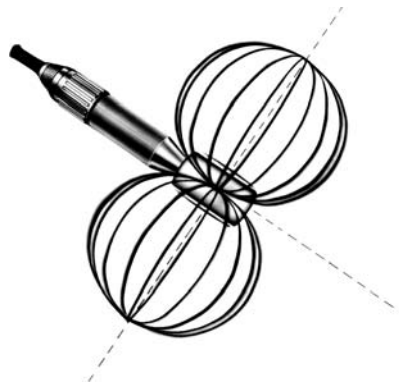
FIGURE 1.5 Bidirectional pickup pattern. Courtesy Sennheiser Electronic Corporation.
