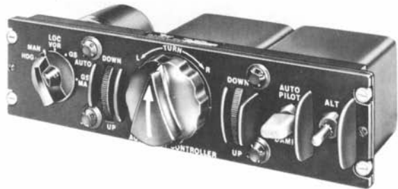
Figure 22.10 Control panel for PB-20D afcs.
