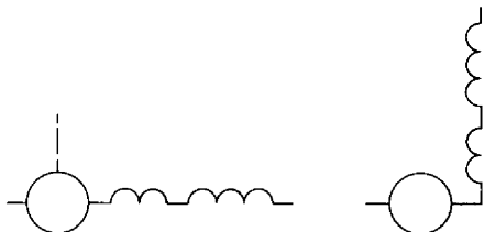
SERIES MOTOR OR 2-WIRE DC GENERATOR WITH COMMUTATING FIELD WINDING OR BOTH
