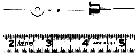
Figure 4.34 Components of a silicon diode rectifier.
