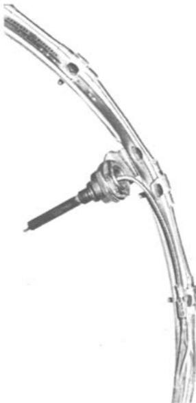
Figure 15.15 Thermocouple unit for jet-exhaust temperature indicator.
