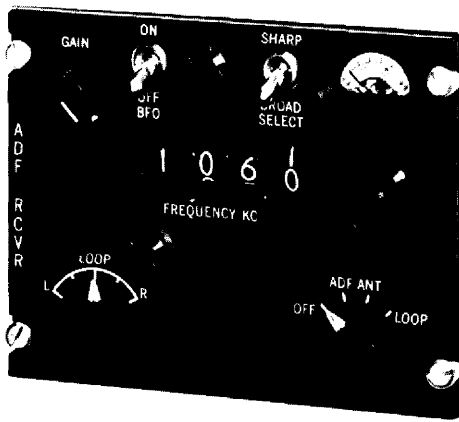
Figure 20.10 Control panel for adf.
