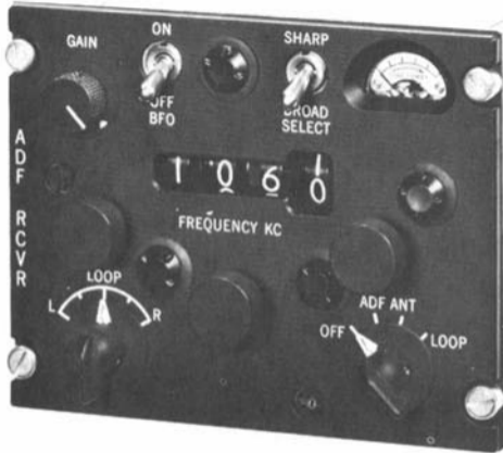
Figure 20.10 Control panel for adf.
