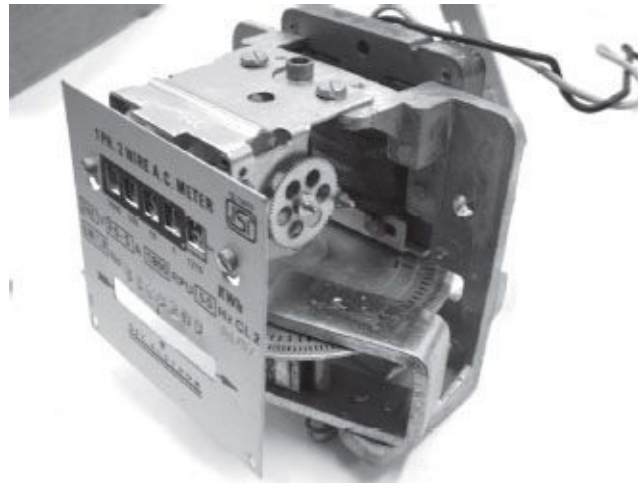
Figure 8.5 Photograph of dial-type single phase energy meter
