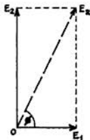
Fig. 132 Phasor representation of voltages E_1 and E_2 and their resultant E_R .
