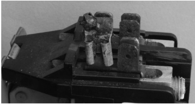
FIGURE 4-4 Overheating caused by a poor connection.
