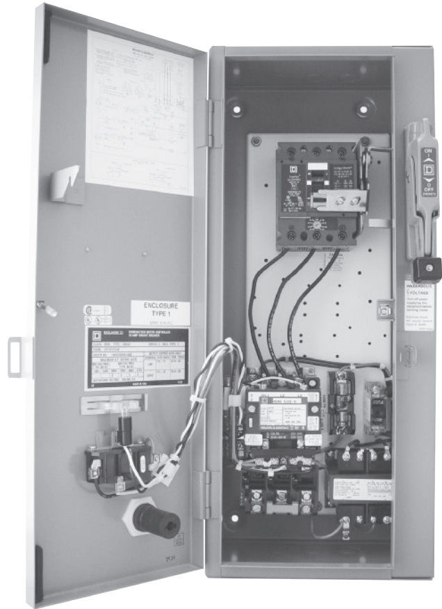
FIGURE 8-9 Combination starters contain the fused disconnect or circuit breaker, control transformer, and motor starter in one enclosure.
