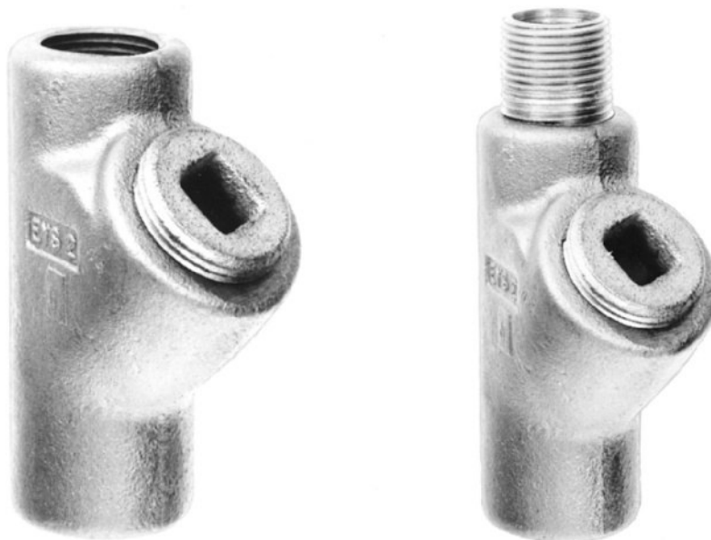
FIGURE 19-5 Seals designed to be installed in the vertical position: used in Class I, Groups A, B, C, D; and Class II, Groups E, F, G.
